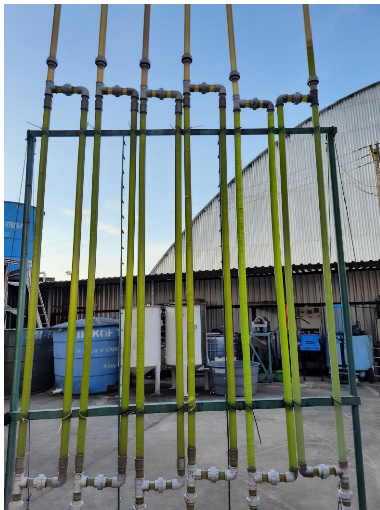
Figure 1. FBR Airlift for microalgae cultivation.
