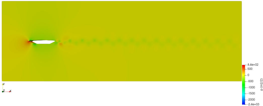
Figure 10. Pressure field for the flow around the Great Belt East Bridge at time t = 30 s.
