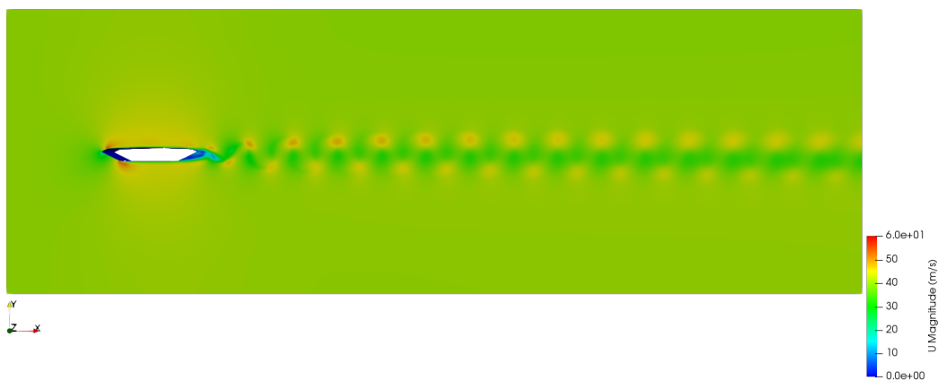
Figure 9. Velocity field for the flow around the Great Belt East Bridge at time t = 30 s.
