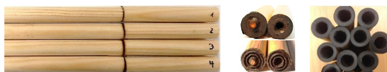
Figure 8. Friction welded wooden bars (left), cross-section surface after tensile break of wood (middle), bamboo (right).
