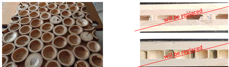
Figure 4. Structure of central layer in CCLT (left) and 3- or 5-layered samples with cover layers of wood.
