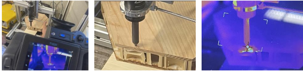
Figure 17. Principle tests for inspection task 3 of Tab. 1 for failure type “crack”: test setup and result image after ultrasonic excitation – the crack in the wood top layer is becoming clearly apparent in the infrared image.
