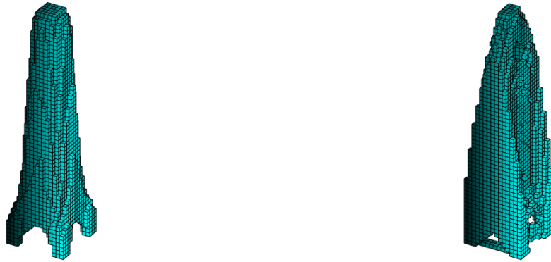
Figure 6: Optimized topology for the tower under (a) vertical and (b) horizontal load.
