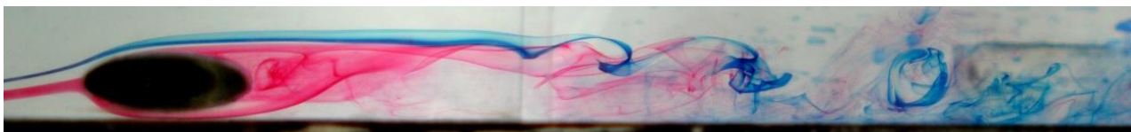
Figure 8. Flow around the cylinder elliptical GR = 0.2 with AR = 0.33 , for Reynolds number of 812, showing vortex appearing and destruction
