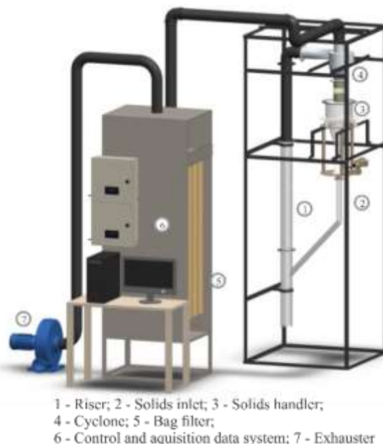
Figure 1. Lab scale circulating fluidized bed unit.
