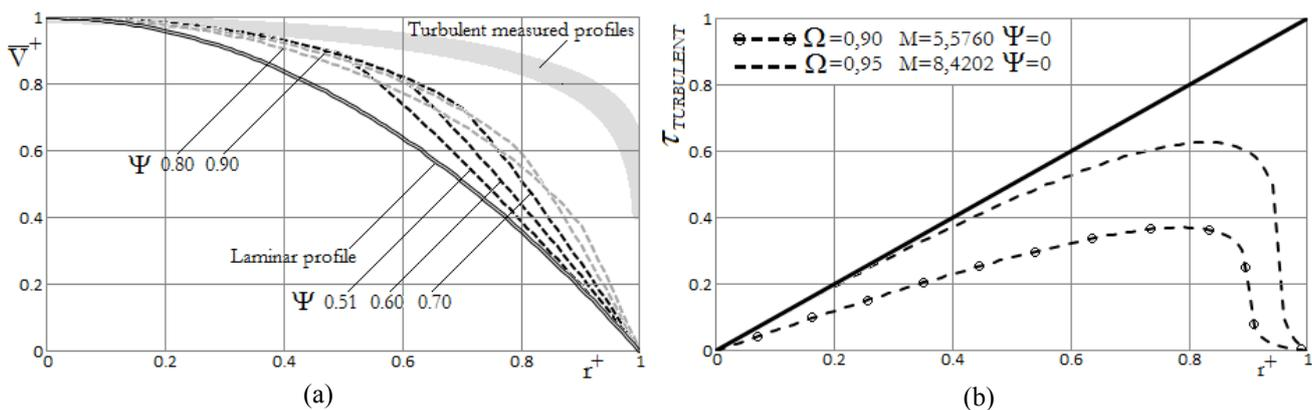
Figure 4. (a) Continuous line: parabolic laminar velocity profile. Dashed lines: profiles of equation (13) for  $\Omega=0$  and  $\Psi$  indicated in the figure. Gray cloud: envelope region of turbulent profiles, according to Hughes and Brighton (1967); (b) Continuous line: total shear stress. Dashed lines: “turbulent” shear stresses calculated with equations (16a, b, c). The values of the parameters  $\Psi$ ,  $\Omega$  and  $M$  are indicated in the figure.
