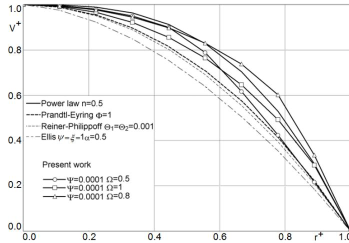
Figure 3. Comparison of the dimensionless velocity profiles and shear stress between the non-Newtonian models of Table 1 and the present approximation.
