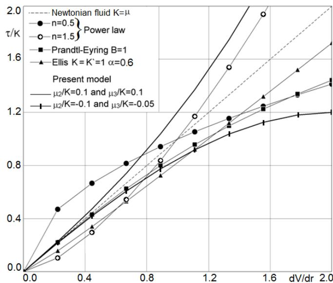
Figure 2. Sketches of the models presented in Table 1 and the present approximation, showing that the present model allows representing pseudoplastic and dilatant fluids for a tange of  $dV/dr$  values.
