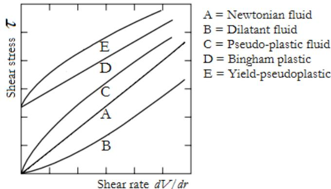
Figure 1. General definition of non-Newtonian fluids accordingly the behavior of the shear stress with the shear rates.
