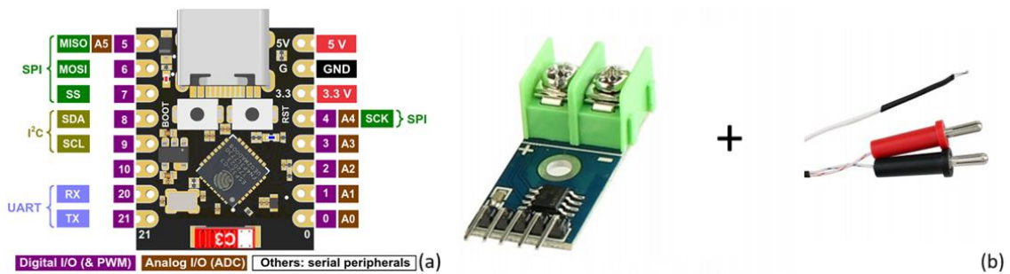
Figura 5. Aparato experimental, (a) ESP-32 C3 Super Mini, (b) MAX6675 e K TP-01A.
