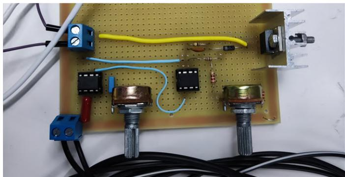
Figura 6. The circuit prototype for DC flyback activation.
