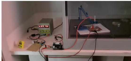
Figura 8. Experimental setup showing the prototype circuit and plasma application to a Petri dish for the characterization of the biocide action.
