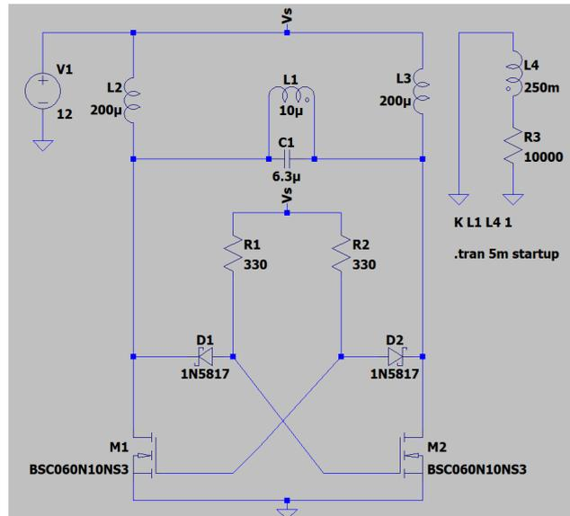
Figura 1. Simplified circuit of the bistable oscillator used for the simulation in LTSPICE. This topology is also known as Zero Volt Switching (ZVS).
