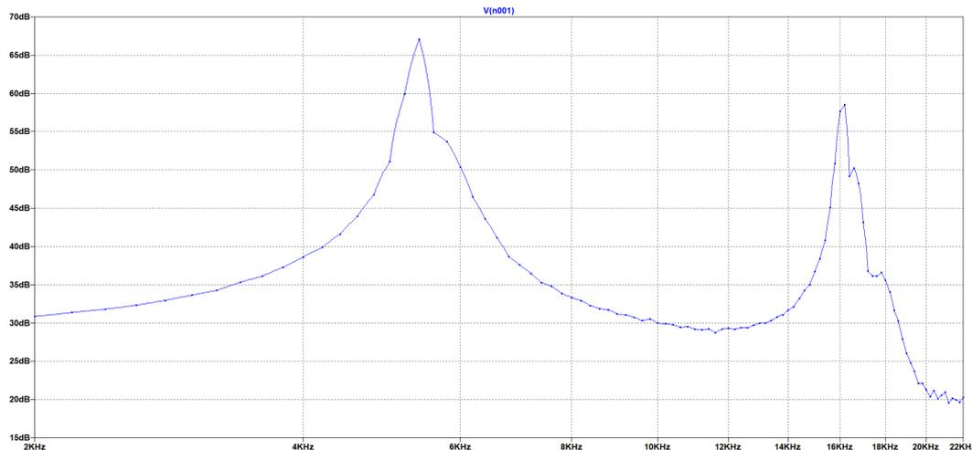
Figura 3. The Fourier power spectrum of the simulated signal at the output. The operating frequency is observed around 5 KHz, which is the resonant frequency for the components in the LC bank.
