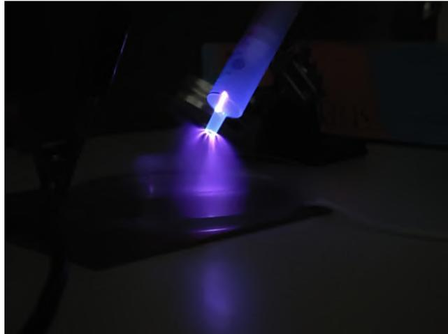
Figura 7. Corona discharge between the electrode inside the syringe and the ground plane.
