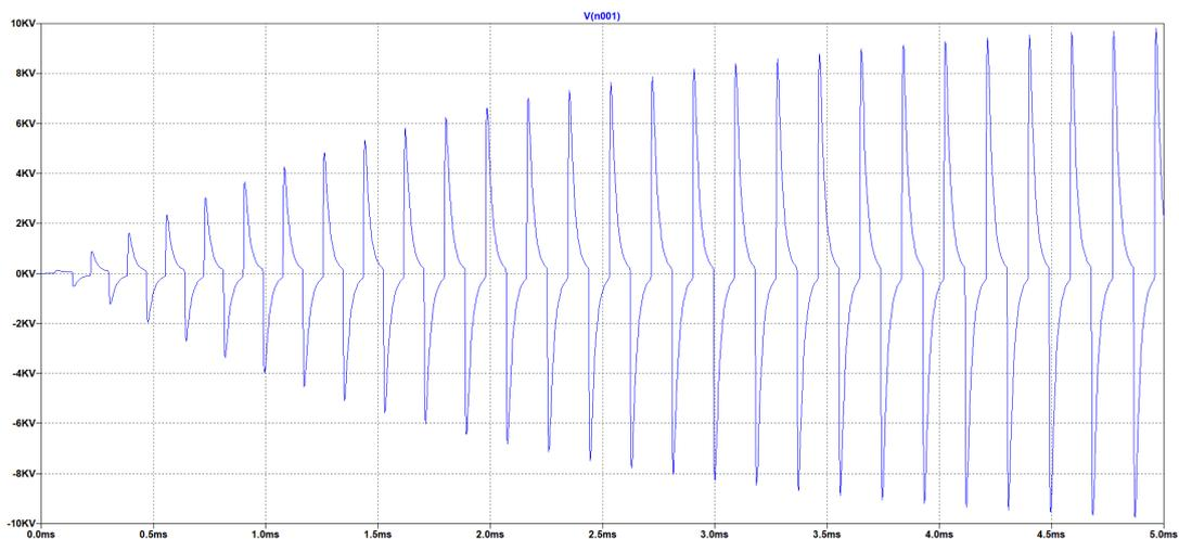
Figura 2. LTSPICE simulation result: It is possible to observe the building up of tension in the output of a flyback transformer. This simulation didn't account for the discharge dynamics of plasma, only the possibility of achieving voltage potentials necessary for gas ionization. This circuit achieve a steady state around 10kV.
