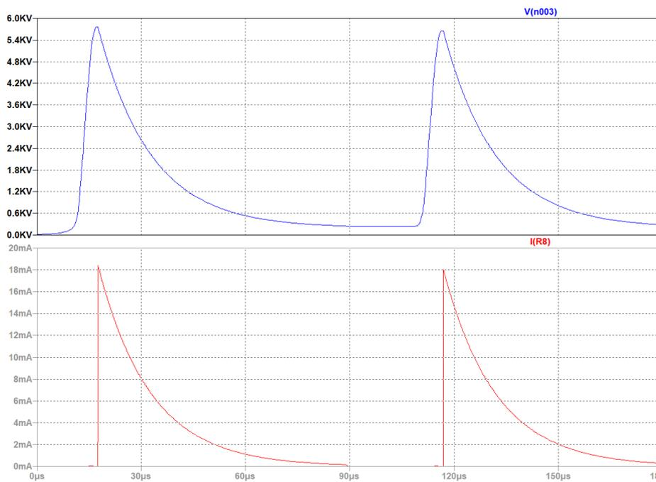
Figura 5. Output signal of the flyback transformer excited by a PWM signal.
