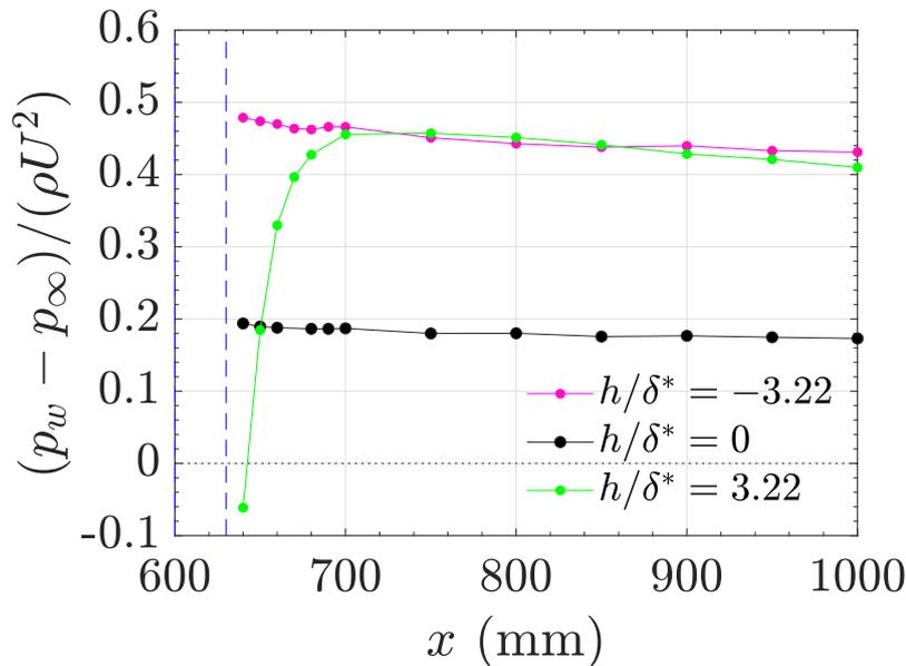
Figure 6: Preston tube data evidencing a backflow region (re-circulation bubble)
