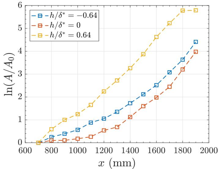
Figure 4: Amplitude ratio between the smooth case, the bump with  $h/\delta^* = 0.64$  and the gap with  $h/\delta^* = -0.64$ .
