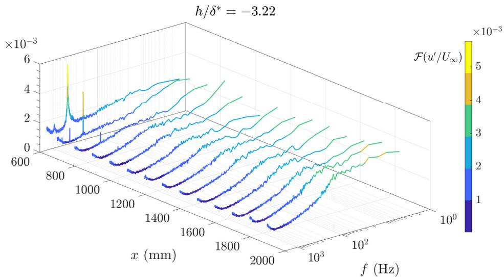
Figure 5: Disturbance velocity evolution along the streamwise direction of the spectrum of the G3 gap case ( $h/\delta^* = -3, 22$ ) exhibiting the presence of the Rossiter mode near the gap.
