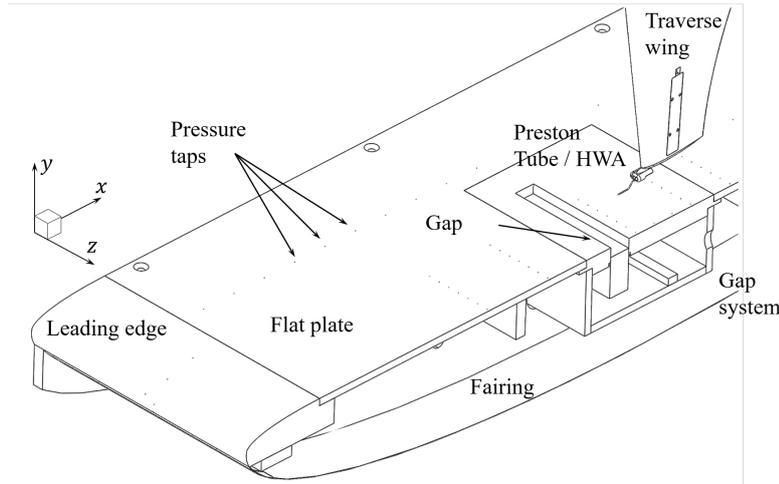
Figure 1: Section view of the model employed in the experiments
