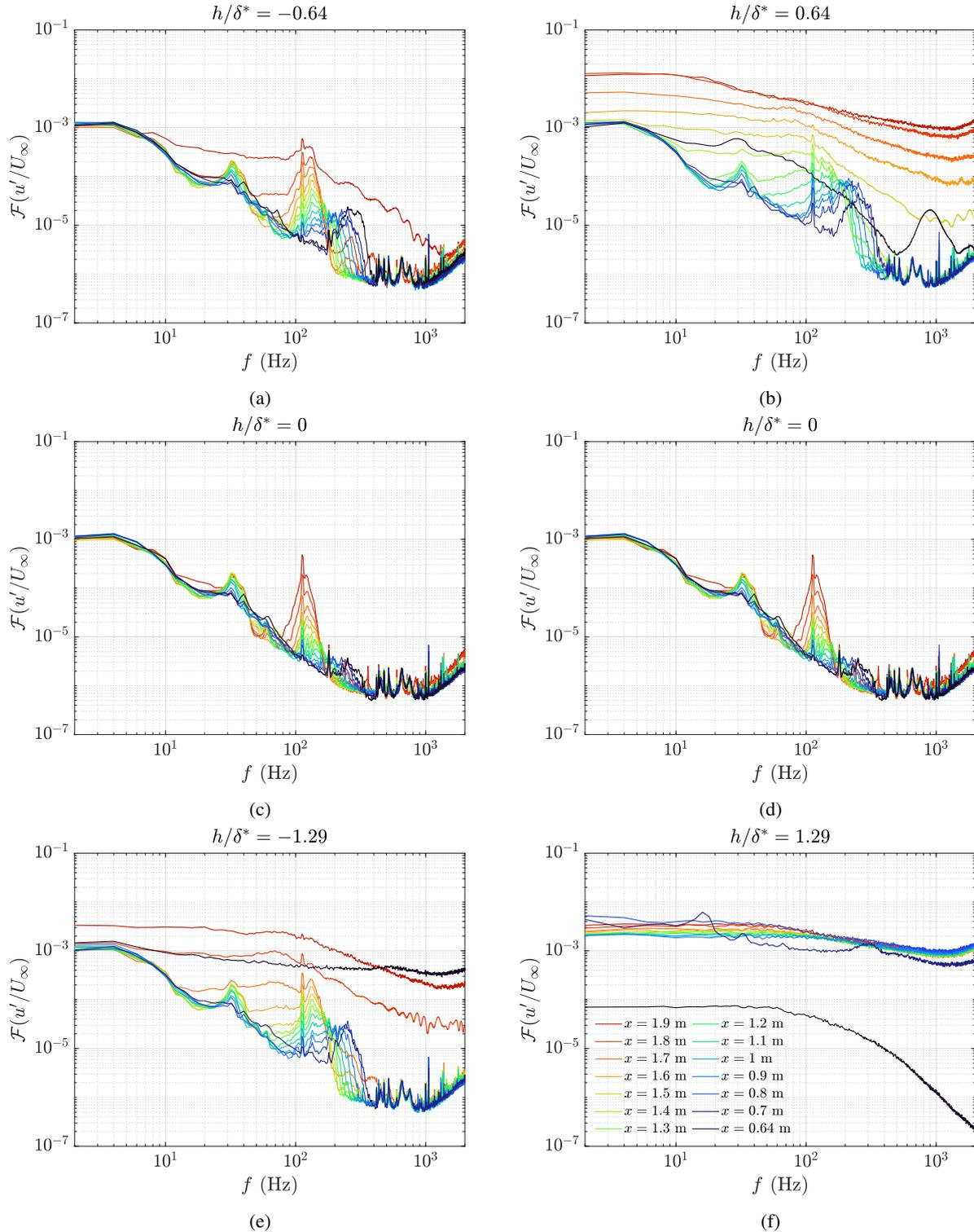
Figure 2: Amplitude of the signals collected by HWA in different configurations of irregularities
