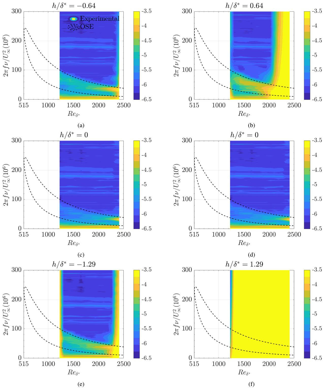
Figure 3: Amplified frequency band in each irregularity configuration compared to the Orr-Sommerfeld equation
