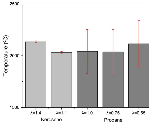
Figure 8. Particle temperature at different stoichiometric ratios.
