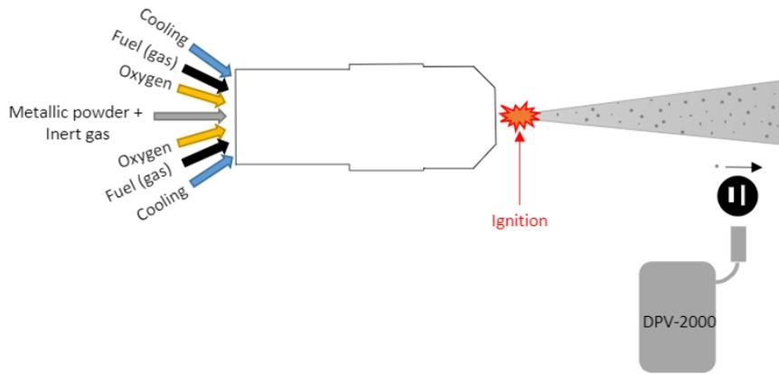
Figure 1. Schematic illustration of the HVOF propane-fueled DJ2700 torch and signal sensing head.
