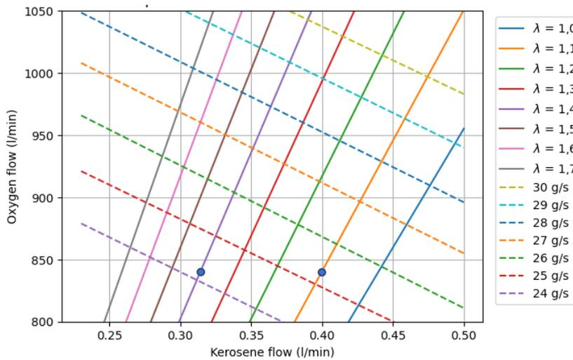
Figure 4. Deposition window of HVOF kerosene-fueled.
