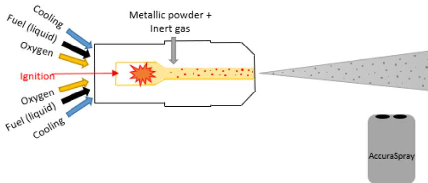
Figure 2. Schematic illustration of the HVOF kerosene-fueled JP5000 torch and signal sensing head.
