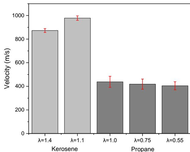
Figure 7. Particle velocity at different stoichiometric ratios.
