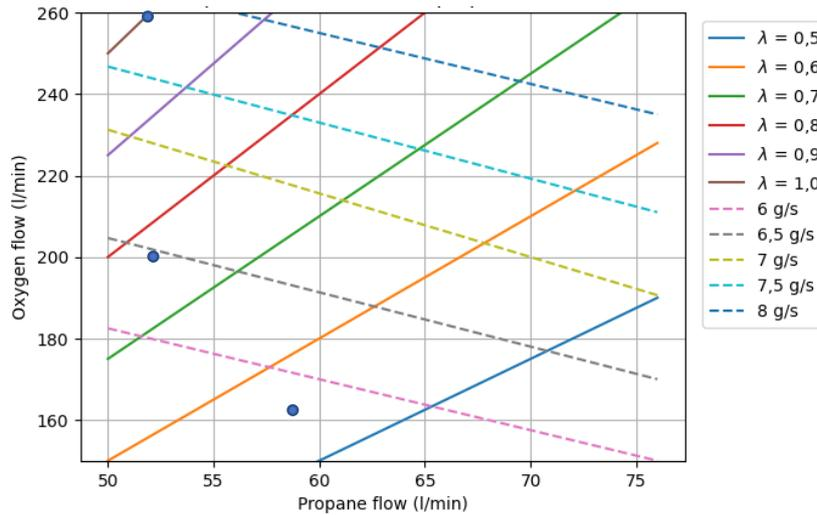
Figure 3. Deposition window of HVOF propane-fueled.
