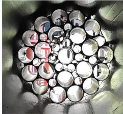
Figure 2. Flow straightener installed in the pipe.
