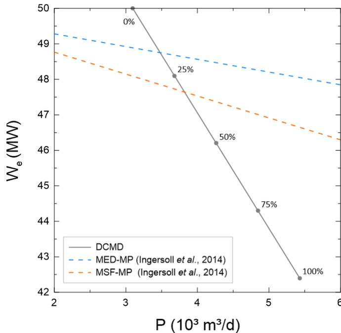
Figure 3. Reactor electrical output  $W_e$  as a function of the total distilled water production  $P$  for different levels of extraction in comparison with other desalination technologies.
