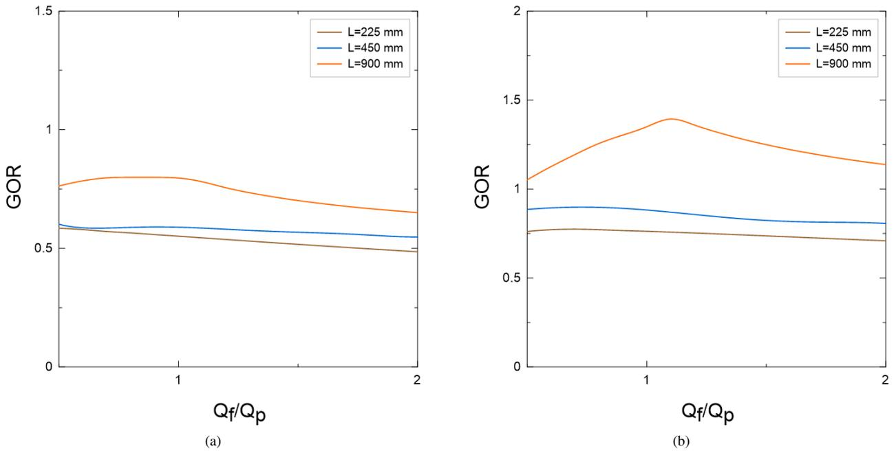
Figure 2.  $GOR$  as a function of the flow rate ratio  $Q_f/Q_p$  for (a) the waste heat recovery plant and (b) the desalination plant with LP steam extraction.
