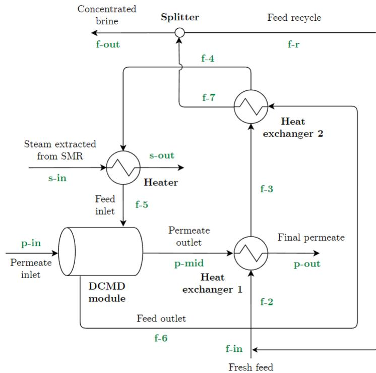
Figure 1. Flow diagram of the desalination plant.
