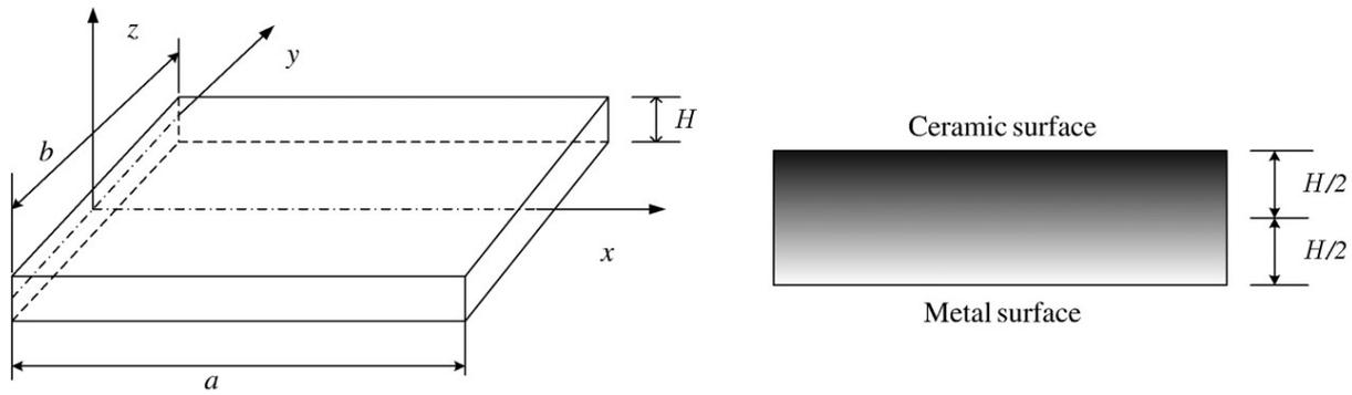
Figure 1. FGM plate's geometry and coordinate system. Source: Lee *et al.* (2010), adapted
