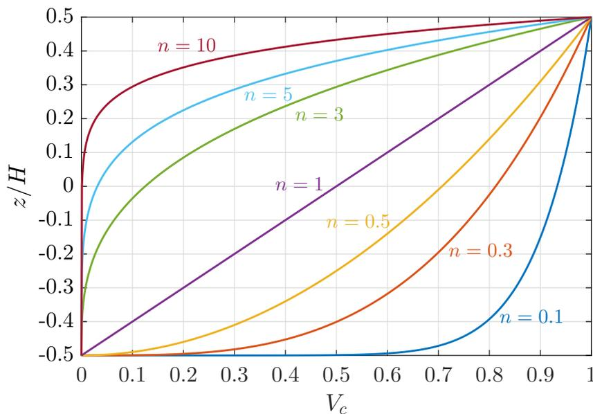
Figure 2. Volumetric fraction of ceramic material along the plate's thickness for different values of  $n$ , showing the distribution parameter's influence on the FGM's composition.
