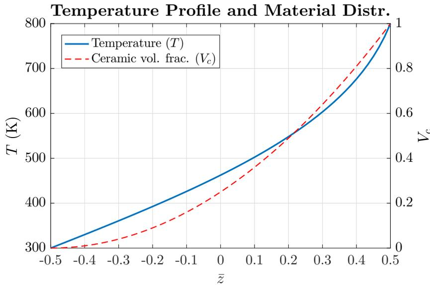
Figure 3. Volumetric fraction of ceramic  $V_c(z)$  and temperature field  $T(z)$  over plate's thickness
