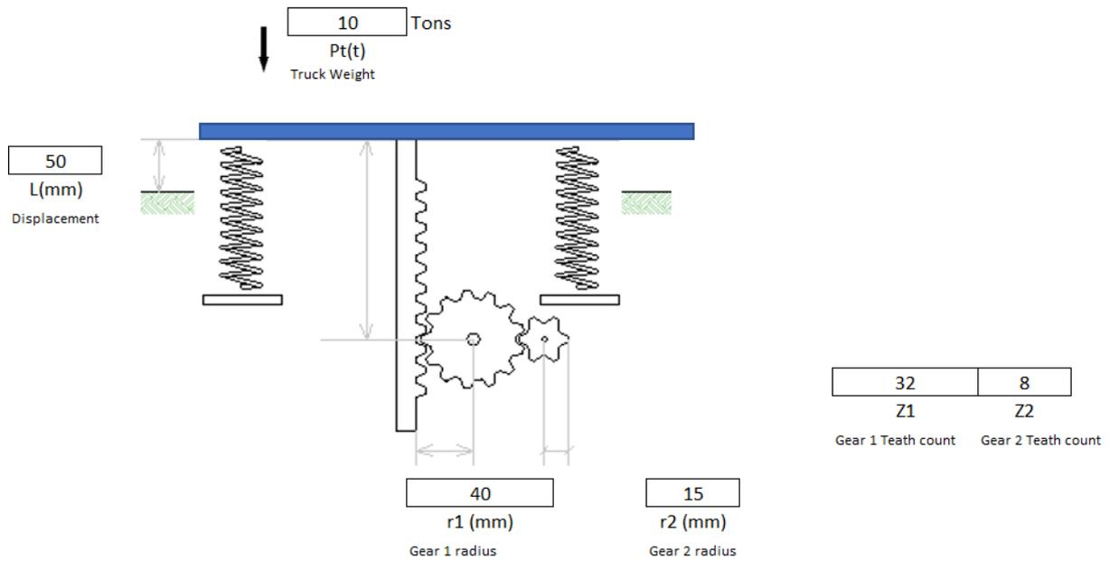
Figure 12. Representation of the mechanical speed bump system.
