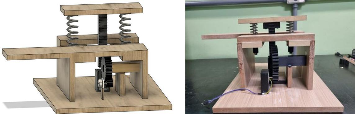
Figure 7. Scaled-down prototype of the mechanical speed bump system.
