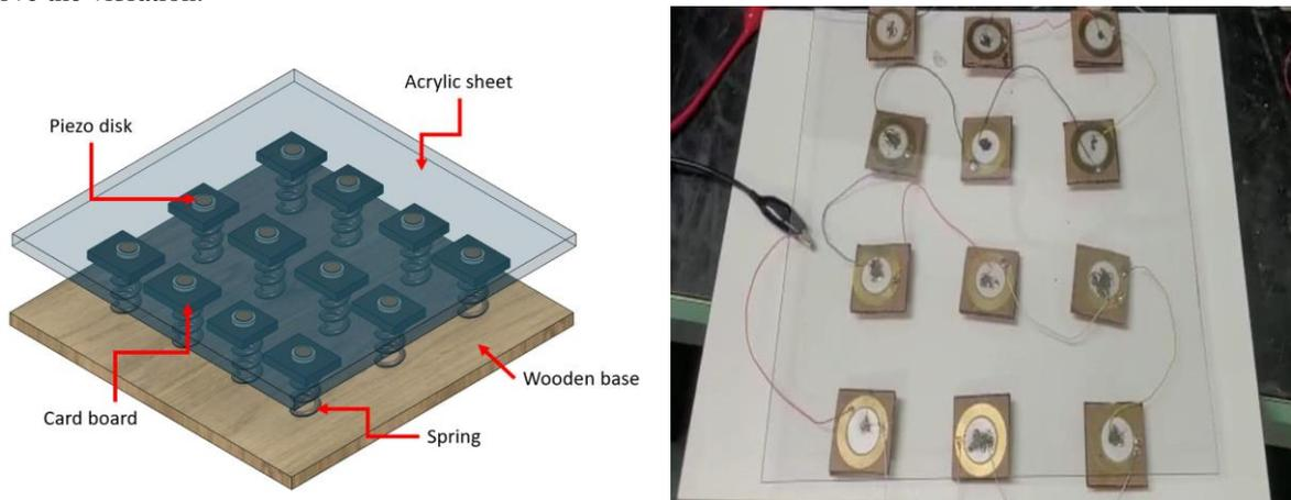
Figure 5. Piezoelectric platform.
