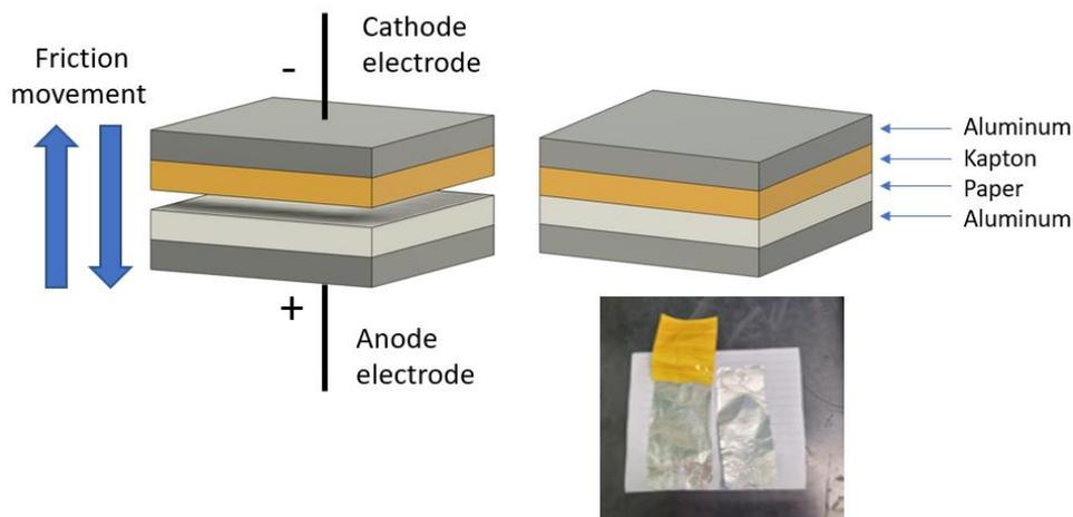
Figure 4. Assembly of the triboelectric system.
