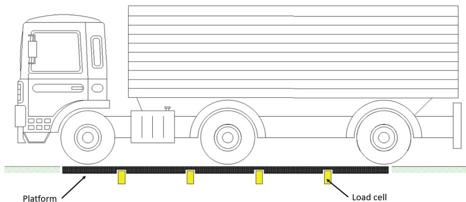
Figure 1. Representation of the truck weighing system.
