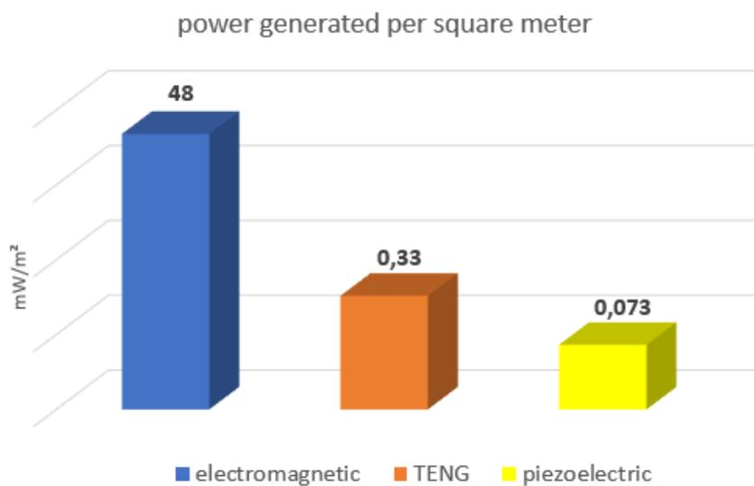
Figure 10. Comparative chart of power generated per square meter.
