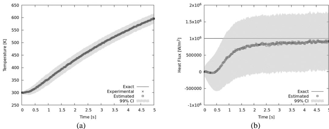
Figure 4. Obtained results for numerical experiment #1 with Kirchoff Transform: (a) temperatures; and (b) heat flux.
