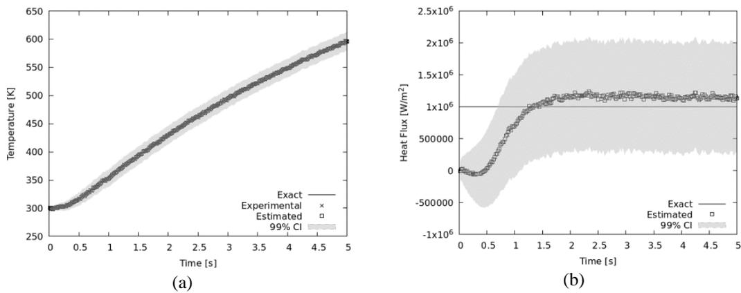
Figure 3. Obtained results for numerical experiment #1 without Kirchoff Transform: (a) temperatures; and (b) heat flux.
