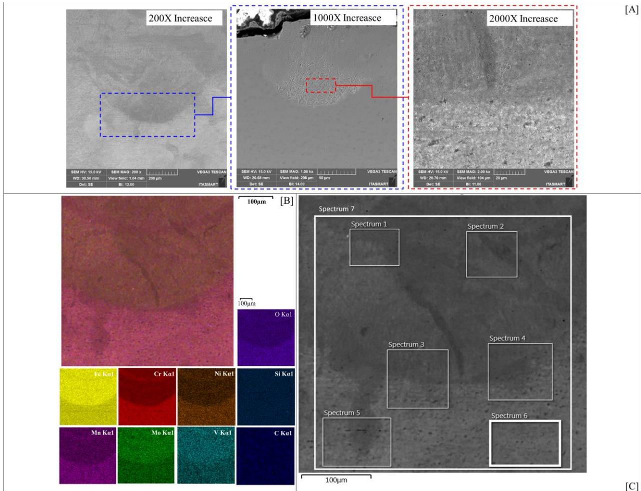
Figure 7. SEM and EDS mapping of *TK-10* track.
