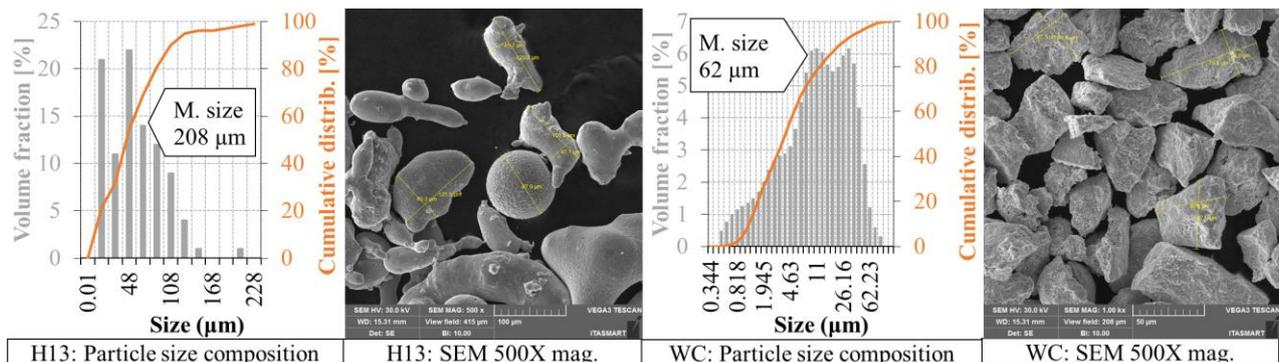
Figure 1. Cladding powders granulometric composition and microstructures.
