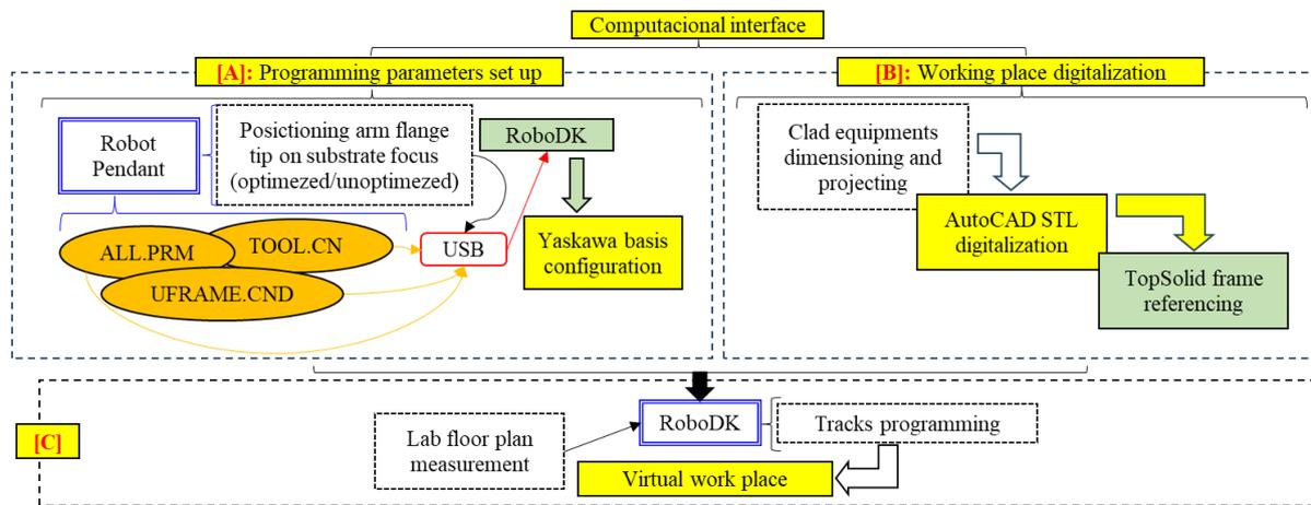
Figure 3. Flowchart of computational interface procedures methods.
