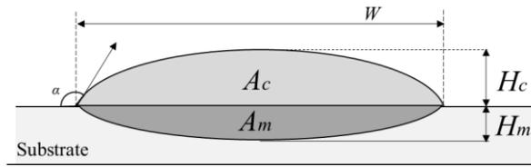
Figure 4. Graphical representation of the cladding variables.
