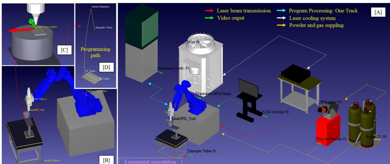
Figure 9. Perspective view of workplace detailing the equipment function and its experiment role.
