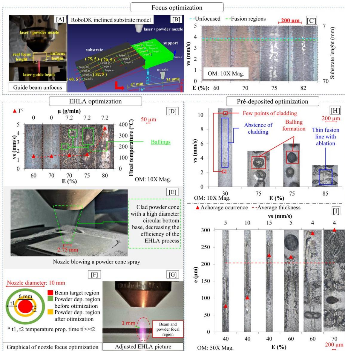
Figure 2. Clad optimization process flowchart.
