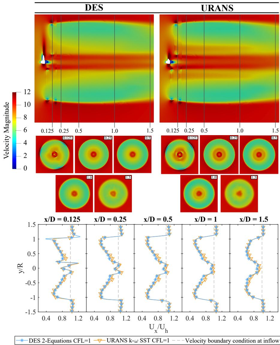
Figure 6: Comparison of the instantaneous wind velocity profiles after 7 complete rotor revolutions at 5  $x/D$  different positions downstream in the wake region along with the iso-contours of the mean velocity field at the same positions for both turbulence models being investigated.
