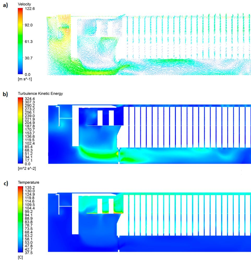
Figure 5. Results in a longitudinal plane of the rotor: a) velocity field; b) turbulence kinetic energy contours; and c) temperature contours.
