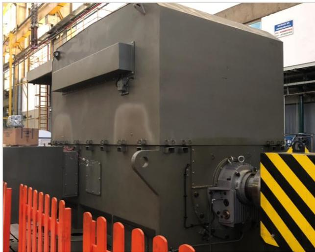
Figure 4. Manufactured turbogenerator.
