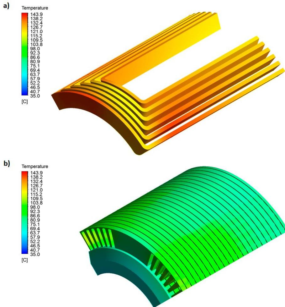
Figure 7. Temperature distribution of the rotor: a) windings; and b) core.
