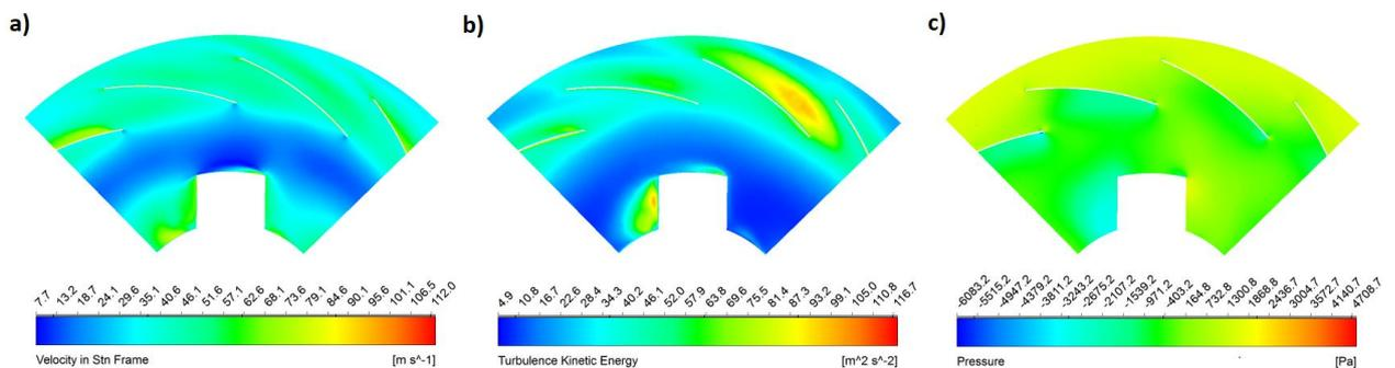
Figure 6. Results in a transversal plane of the fan: a) velocity contours; b) turbulence kinetic energy contours; and c) pressure contours.
