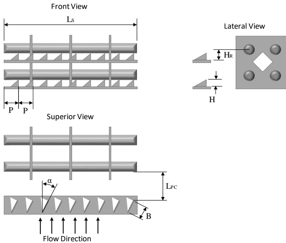
Figure 2. Parameters of the VGs and its assembly in the holding support (Zanatta et al., 2020).
