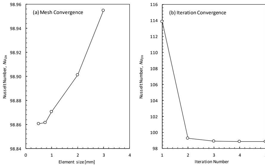
Figure 5. Convergence tests. (a) Mesh convergence and (b) Iteration convergence
