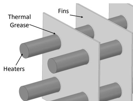
Figure 3. Layer of thermal grease in heat exchanger apparatus.
