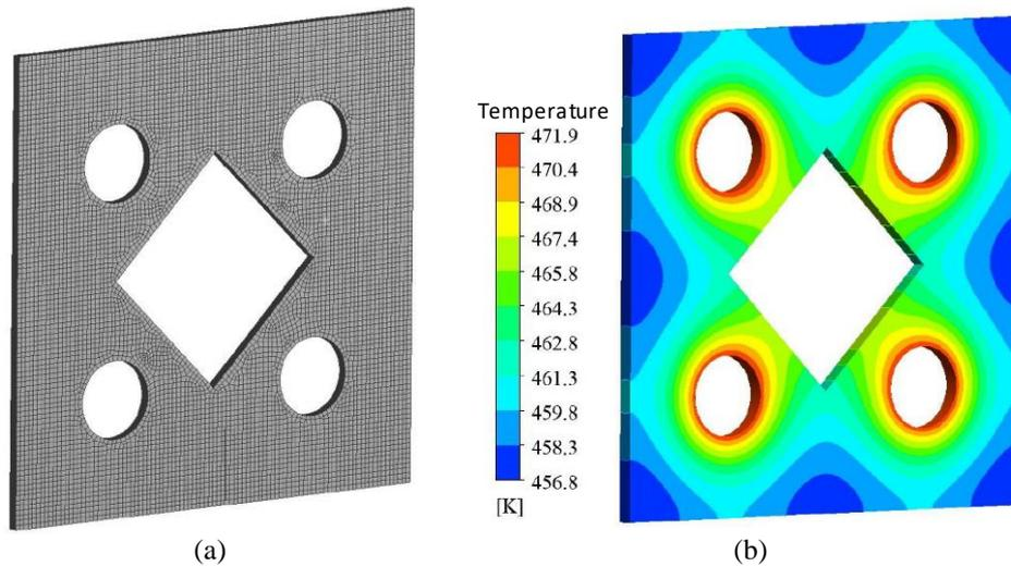
Figure 6. Simulated fin (a) Mesh with 1,0 mm sized elements (b) Temperature distribution.
