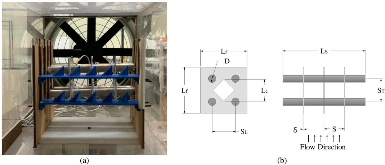
Figure 1. Heat exchanger (a) Assembly of the apparatus and (b) dimensional measures.
