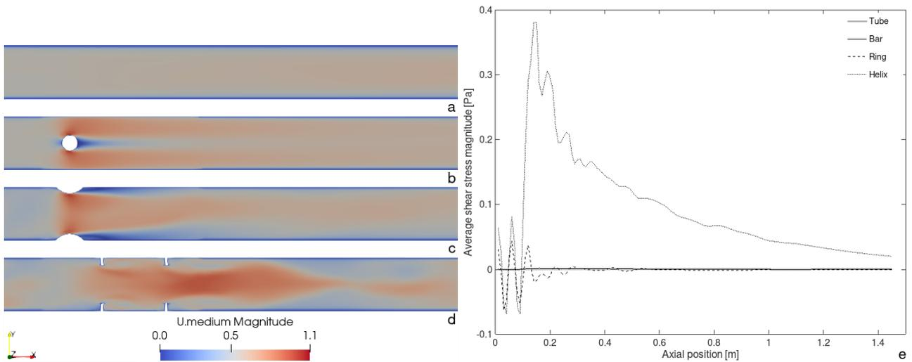
Figure 2. Velocity fields predicted for photobioreactors with (a) smooth tube, and the inclusion of (b) a horizontal bar, (c) a ring, and (d) a helical mixer; (e) swirl number calculated along the length for each configuration.
