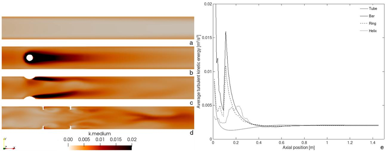
Figure 4. Turbulent kinetic energy predicted for photobioreactors with (a) smooth tube, and the inclusion of (b) a horizontal bar, (c) ring baffle, and (d) a helical mixer; (e) average values calculated along the length for each configuration.
