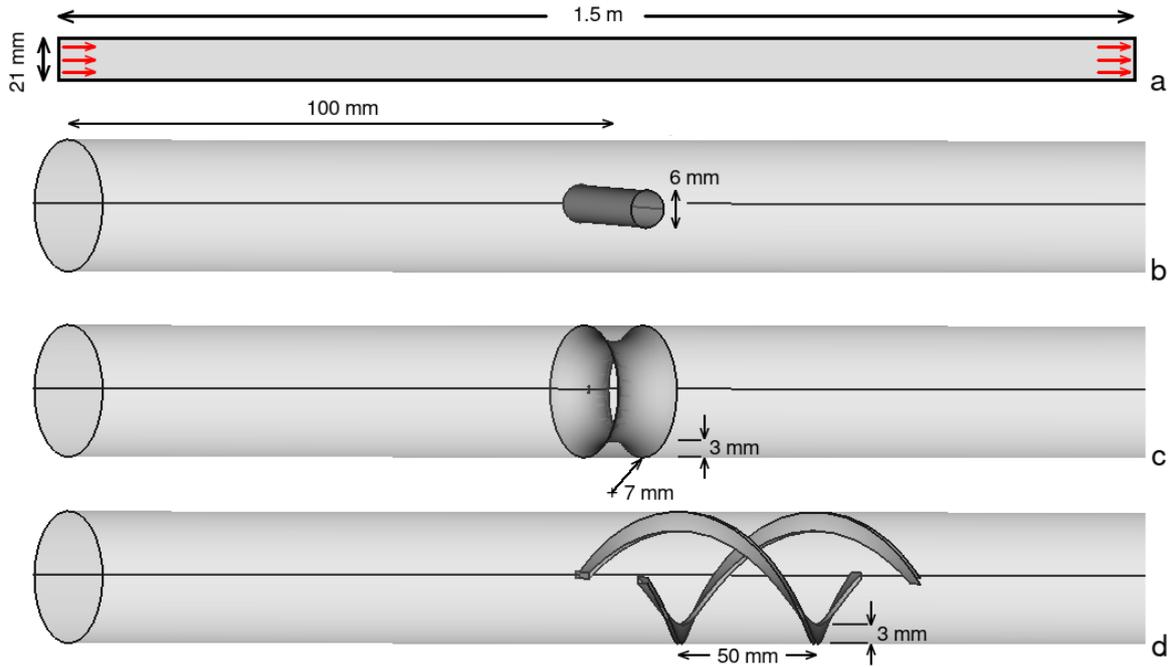
Figure 1. Tubular photobioreactor geometries: (a) smooth tube, (b) horizontal bar, (c) ring baffle, and (d) helical mixer.
