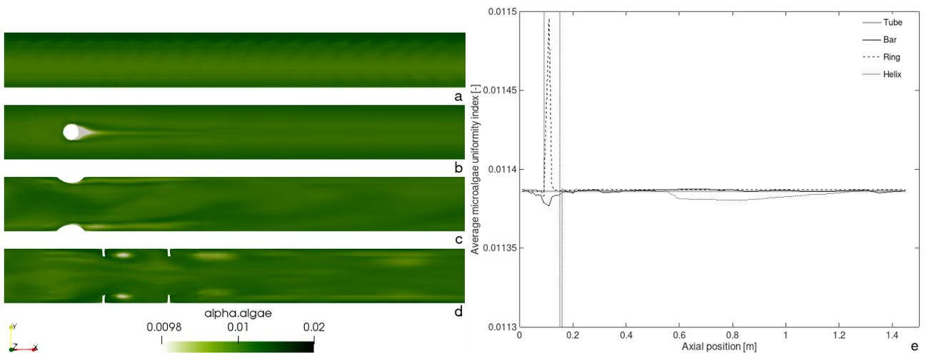
Figure 3. Microalgae volume fraction distribution predicted for photobioreactors with (a) smooth tube, and the inclusion of (b) a horizontal bar, (c) ring baffle, and (d) a helical mixer; (e) uniformity index calculated along the length for each configuration.
