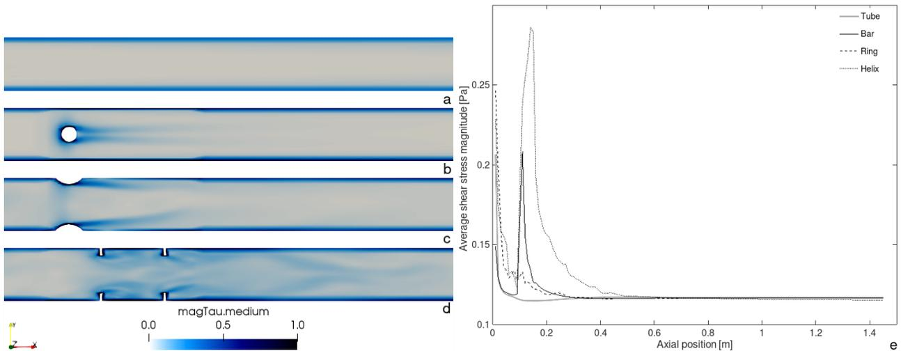
Figure 5. Shear stress predicted for photobioreactors with (a) smooth tube, and the inclusion of (b) a horizontal bar, (c) ring baffle, and (d) a helical mixer; (e) average values calculated along the length for each configuration.
