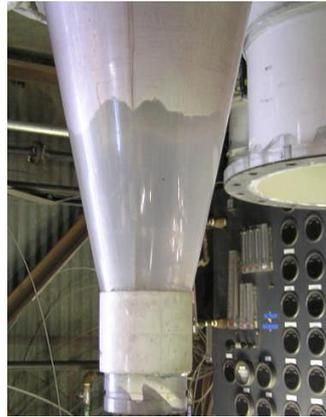
Figure 8. Photograph of Erosion of drywall in the cone of a second-stage Cyclone (Karri et al. (2011)).
