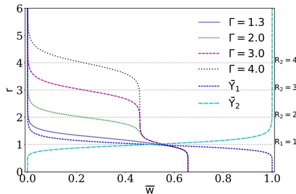
Figure 4. Mass fraction  $\bar{Y}_1$  and  $\bar{Y}_2$  base flow profiles together with base flow axial velocity profiles obtained using different  $\Gamma$  ratios.
