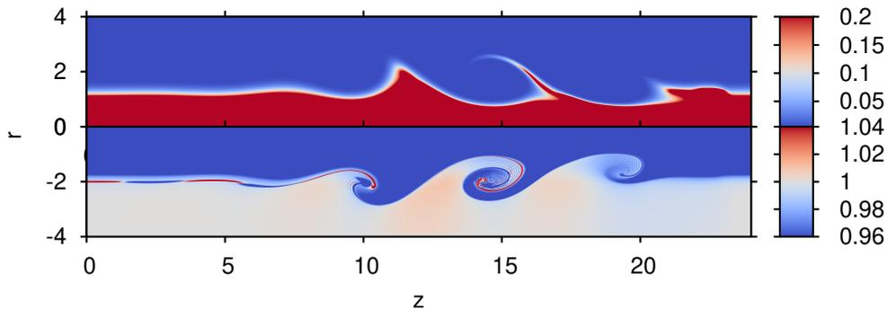
Figure 14. Mass fraction contours and density contours, showing the vortical structures for  $H_2 - O_2$  coaxial jet at  $t = 50$ . Mass fraction contours are shown for  $r > 0$  and density contour for  $r < 0$ . The radii and velocity ratios used were  $\Gamma = 2.0$   $h = 0.5$ , respectively.
