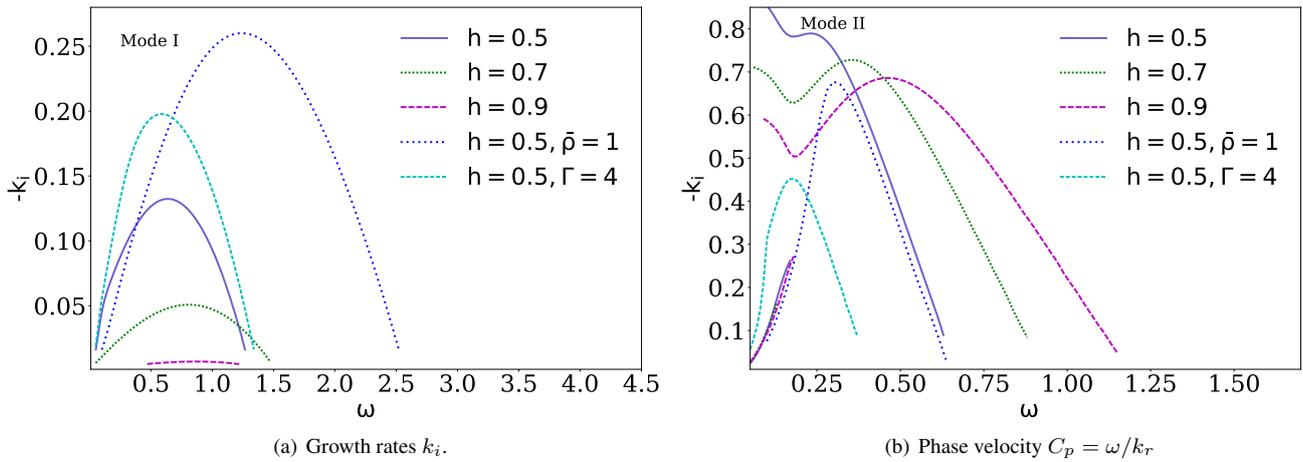
Figure 9. Effect of  $h$  ratio on instability characteristics of the coaxial binary jet configuration  $H_2 - O_2$  with  $\Gamma = 2$ .  $\bar{\rho} = 1$  is the most unstable homogeneous case for Mode I and  $\Gamma = 4$  with  $h = 0.5$  has the most unstable mode I.
