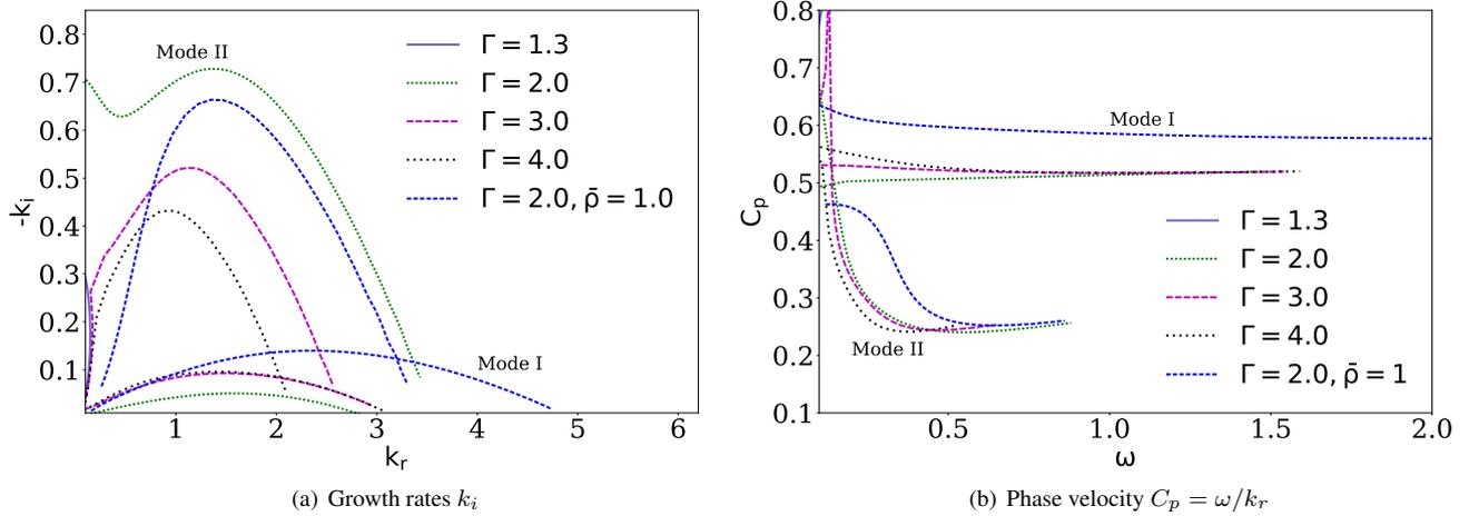
Figure 5. Effect of  $\Gamma$  ratio on instability characteristics of the coaxial binary jet configuration  $H_2 - O_2$  with  $h = 0.7$ .
