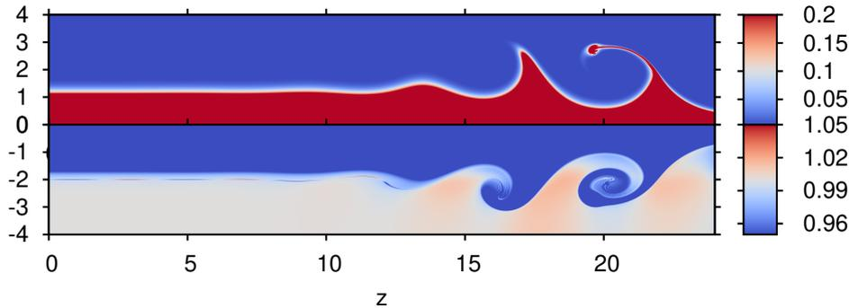
Figure 11. Mass fraction contours and density contours, showing the vortical structures for  $H_2 - O_2$  coaxial jet at  $t = 70$ . Mass fraction contours are shown for  $r > 0$  and density contour for  $r < 0$ . The radii and velocity ratios used were  $\Gamma = 2$   $h = 0.7$ , respectively.
