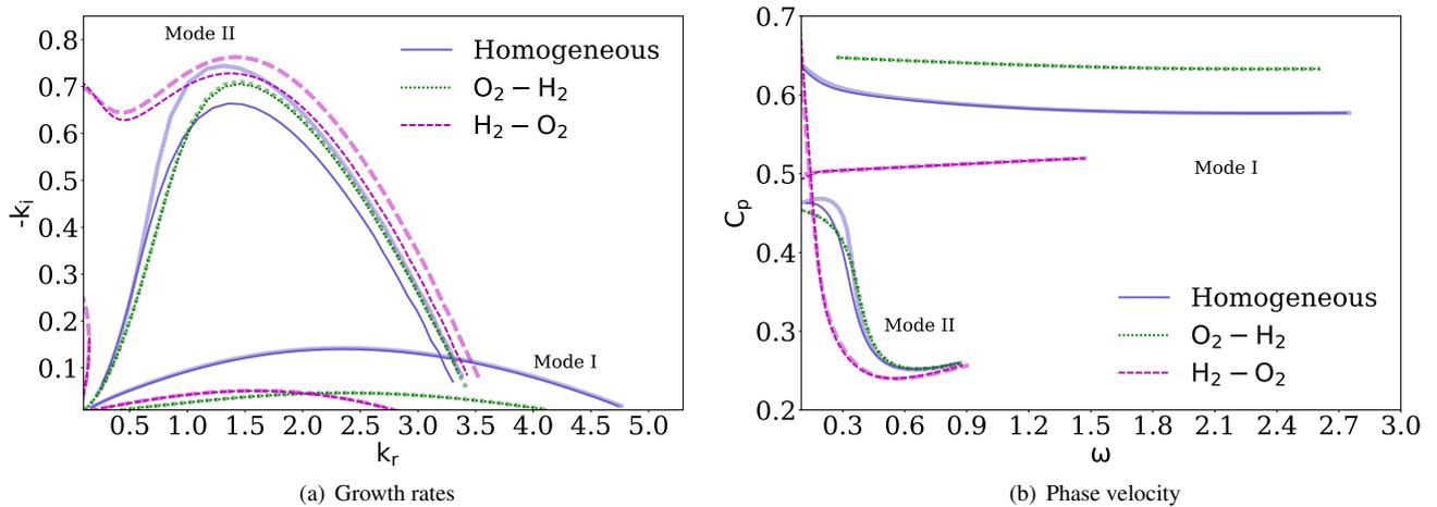
Figure 3. Effect of species configuration and compressibility (thinner lines) on the coaxial jet Modes growth rates ( $-k_i$ ) and on phase velocity  $C_p$ . With  $\Gamma = 2$  and  $h = 0.7$ .
