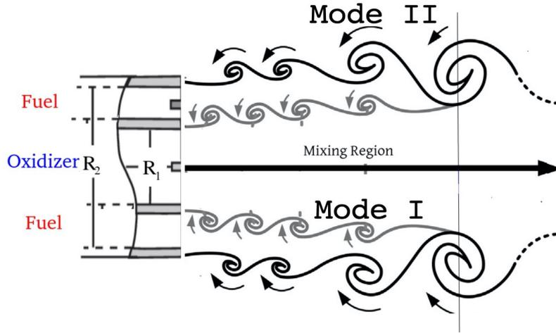
Figure 1. Mixing process between oxidizer and fuel in a shear coaxial injector produced by the Kelvin-Helmholtz instability.
