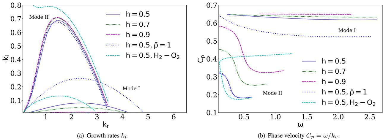
Figure 10. Effect of  $h$  on instability characteristics of the coaxial binary jet configuration  $O_2 - H_2$  with  $\Gamma = 2$ .  $\bar{\rho} = 1$  is the most unstable homogeneous case for Mode I, and  $H_2 - O_2$  case with  $h = 0.5$  is the most unstable mode.
