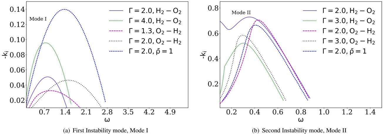
Figure 7. The most relevant cases evaluated to illustrate the effect of  $\Gamma$  ratio on of the growth rate and phase velocity of coaxial binary jets with  $h = 0.7$ .
