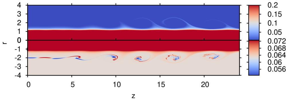
Figure 15. Mass fraction contours and density contours, showing the vortical structures for  $O_2 - H_2$  coaxial jet at  $t = 70$ . Mass fraction contours are shown for  $r > 0$  and density contour for  $r < 0$ . The radii and velocity ratios used were  $\Gamma = 2.0$   $h = 0.5$ , respectively.
