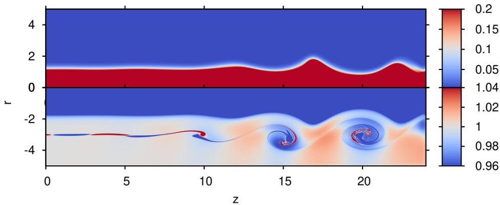
Figure 13. Mass fraction contours and density contours, showing the vortical structures for  $H_2 - O_2$  coaxial jet at  $t = 70$ . Mass fraction contours are shown for  $r > 0$  and density contour for  $r < 0$ . The radii and velocity ratios used were  $\Gamma = 3$   $h = 0.7$ , respectively.
