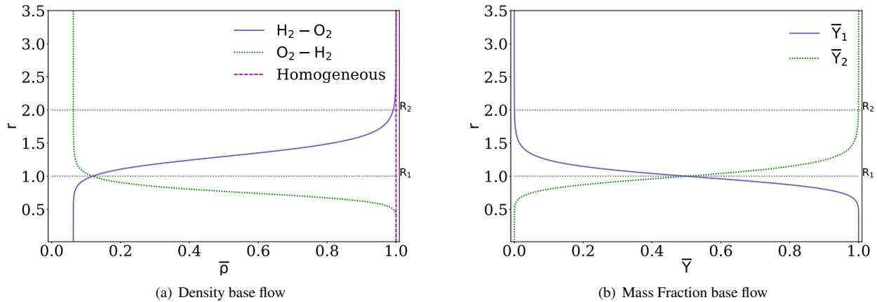
Figure 2. Density base flow and Mass fraction profiles for different binary coaxial jets, non-dimensionalized with respect to the oxygen jet at the  $r = 0$  temperature,  $\Gamma = 2$  and  $h = 0.7$ .
