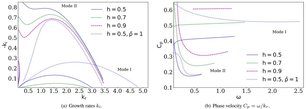
Figure 8. Effect of  $h$  ratio on instability characteristics of the coaxial binary jet configuration  $\text{H}_2 - \text{O}_2$  with  $\Gamma = 2$ .  $\bar{\rho} = 1$  is the most unstable homogeneous case for Mode I.
