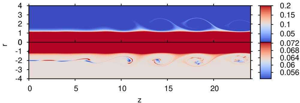
Figure 12. Mass fraction contours and density contours, showing the vortical structures for  $O_2 - H_2$  coaxial jet at  $t = 70$ . Mass fraction contours are shown for  $r > 0$  and density contour for  $r < 0$ . The radii and velocity ratios used were  $\Gamma = 2$   $h = 0.7$ , respectively.
