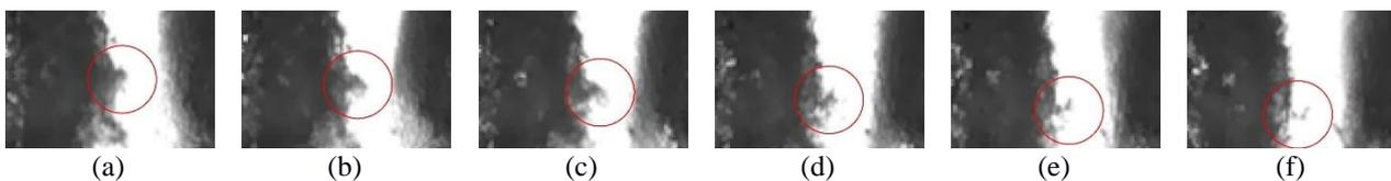
Figure 8. Droplet formation on Region C with a timestep of  $1.72 \times 10^{-5}$  s between snapshots.
