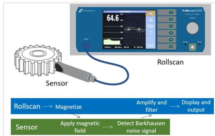
Figure 1. Schematic diagram of the equipment used (adapted from Heiskanen, 2019).
