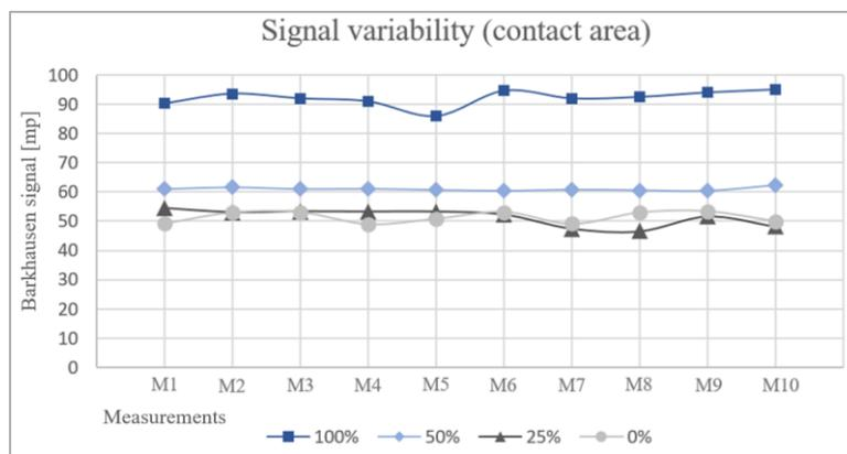
Figure 9. Analysis of signal variation as a function of the magnetic *Barkhausen* noise sensor contact area.
