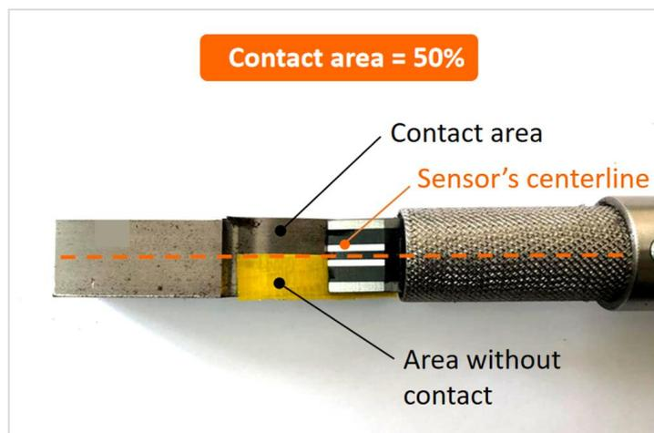
Figure 4. Schematic diagram of measurements as a function of the contact area.
