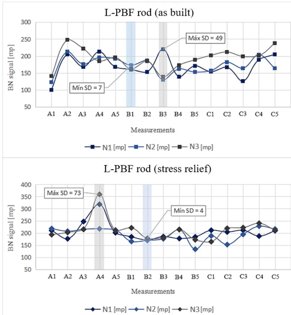
Figure 6. Results of the magnetic *Barkhausen* noise sensor measurements in the L-BPF rod samples (as built and stress relief).
