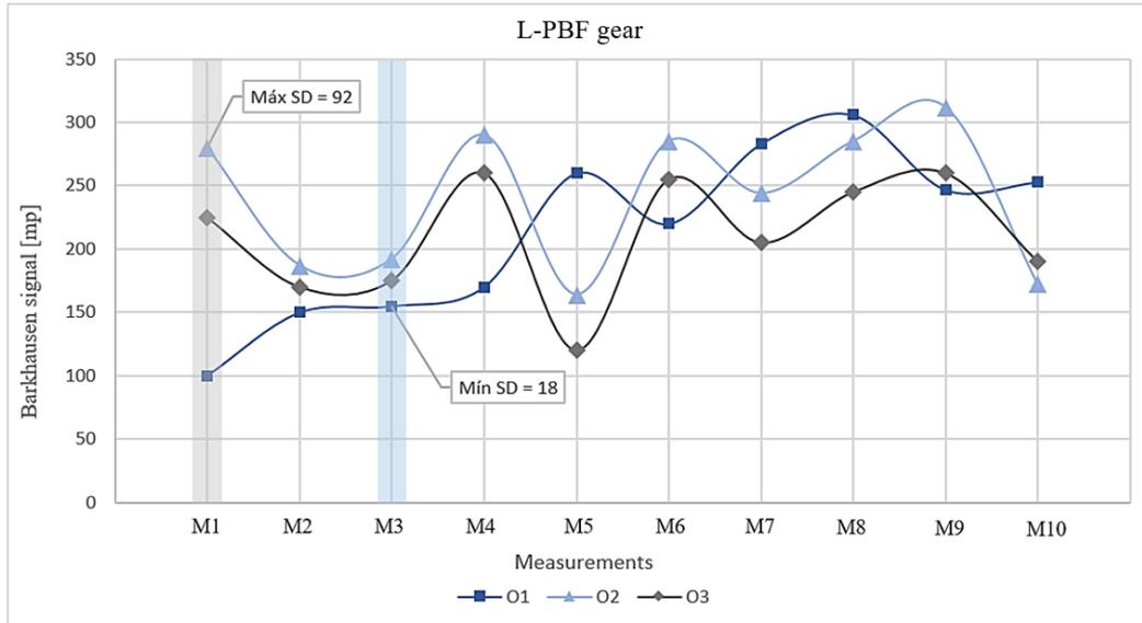
Figure 7. Results of the magnetic Barkhausen noise measurements in the L-PBF gear. The letter “O” stands for "operator" (O1, operator 1) and M for measurement (M1, measurement 1).
