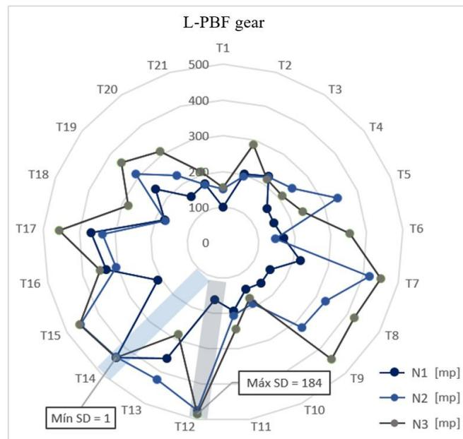
Figure 5. Results of the L-PBF gear measurements with the magnetic *Barkhausen* noise sensor.
