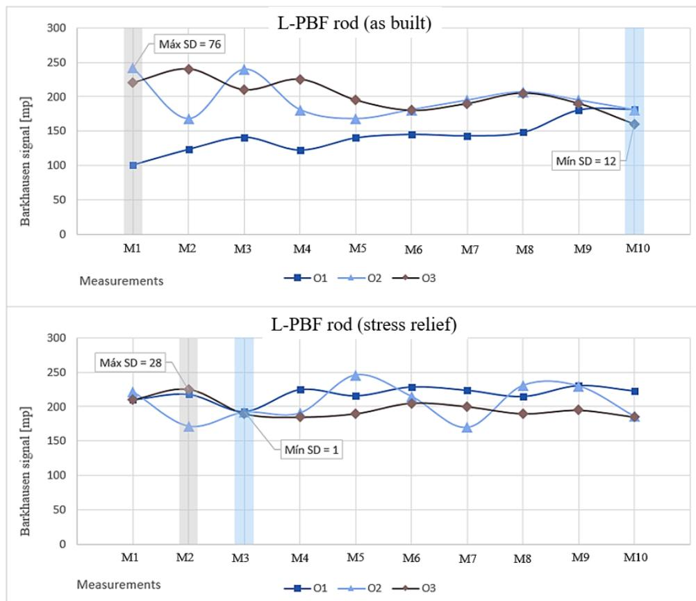
Figure 8. L-PBF rods (as built and stress relief) measurement results. The letter “O” stands for "operator" (O1, operator 1) and M for measurement (M1, measurement 1).
