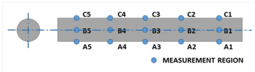
Figure 3. Schematic diagram of the measurement regions in the L-BPF rod samples.
