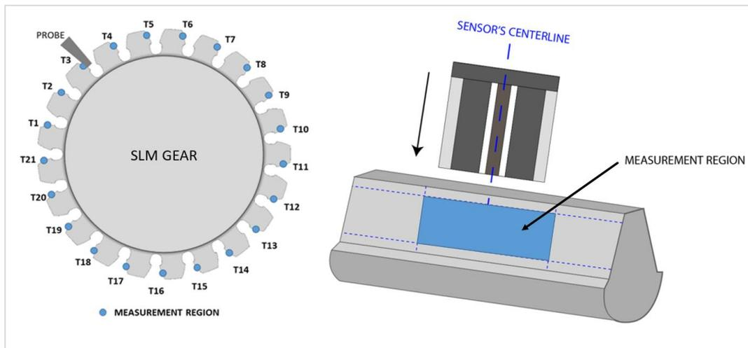
Figure 2. Schematic diagram of the measurement regions in the sample L-PBF gear
