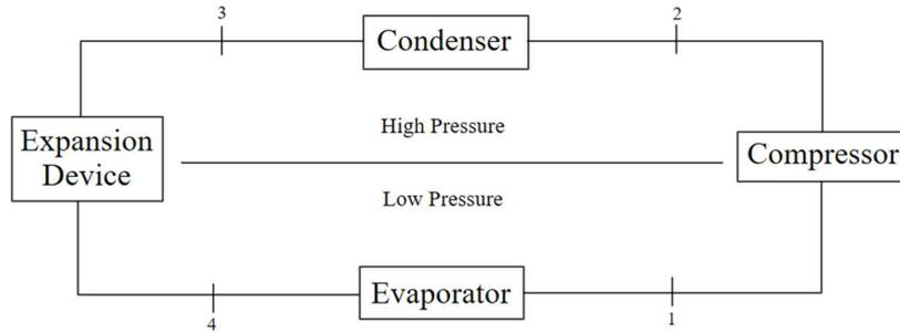
Figure 1. Diagram of a vapor compression cycle.
