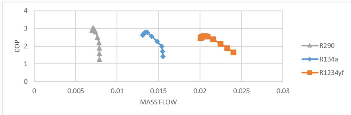
Figure 3. Simulation result for ambient temperature equal 35°C.
