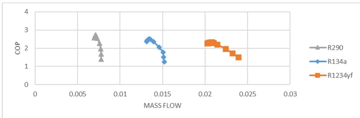
Figure 4. Simulation result for ambient temperature equal to 40°C.
