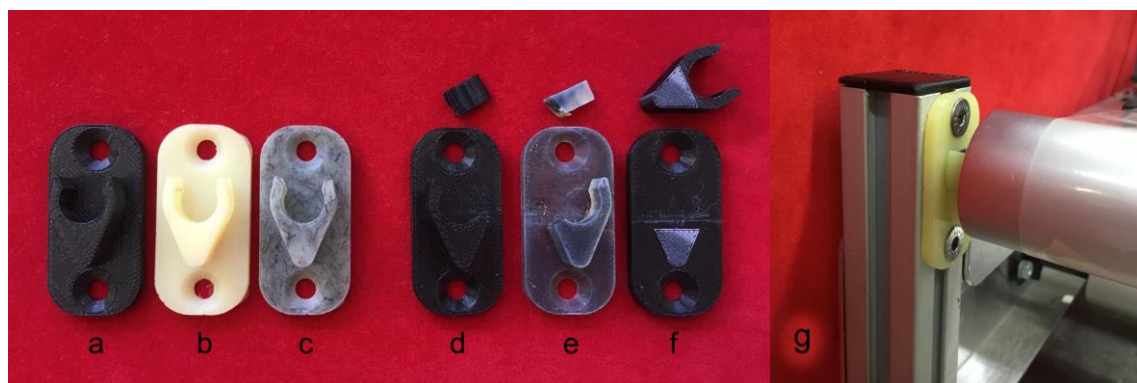
Figura 8. Suportes fabricados nos materiais: (a) ABS; (b) C; (c) F; (d) ABS; (e) B; (f) ABS; (g) E
