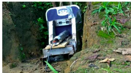
Figure 10. SELENE’s rocket motor static fire test platform
