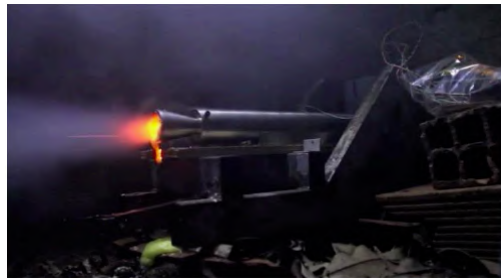
Figure 12. Static Fire Test with bad combustion
