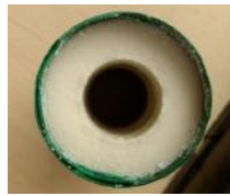
Figure 4. Grain after the casting process, with a visible green inhibitor
