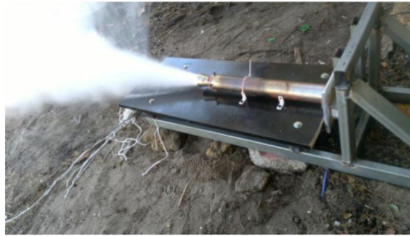
Figure 14. Static fire test of the rocket motor of SELENE
