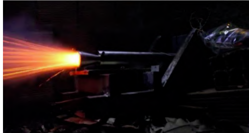
Figure 11. Static Fire Test in the beginning of the combustion
