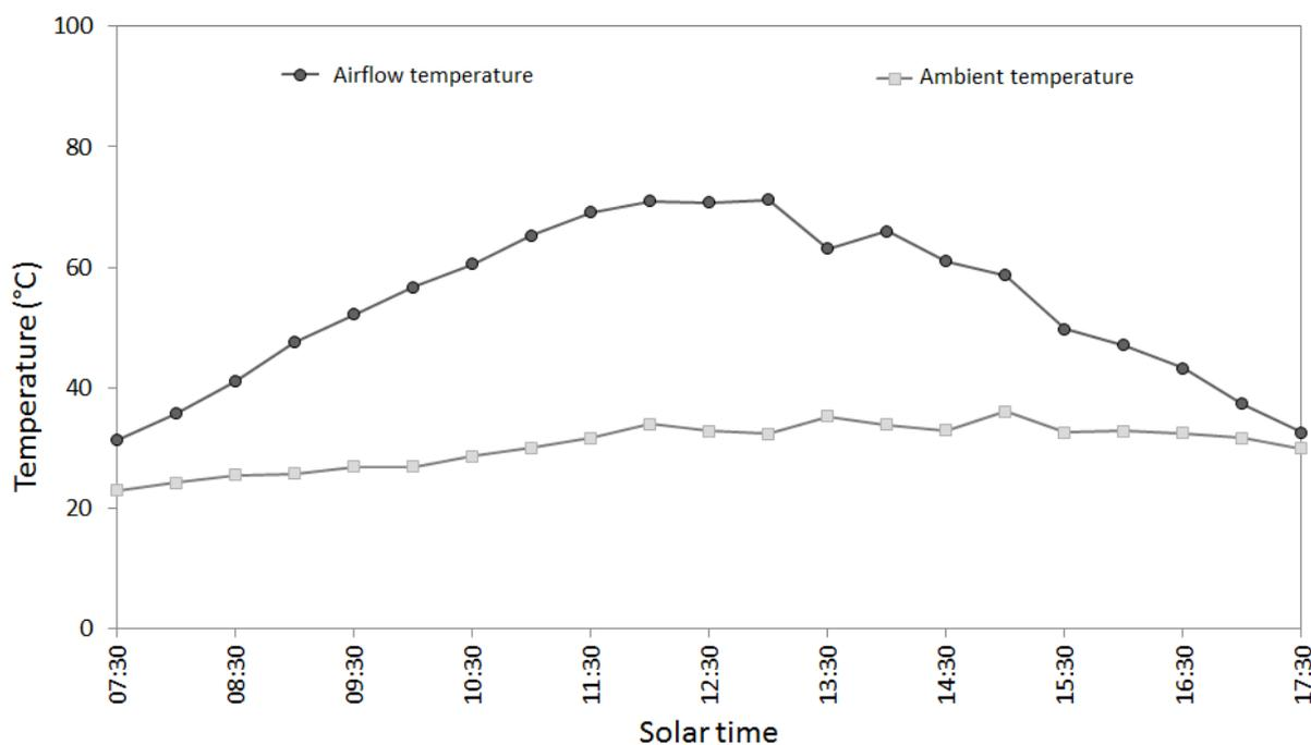
Figure 5. Drying temperature and ambient temperature
