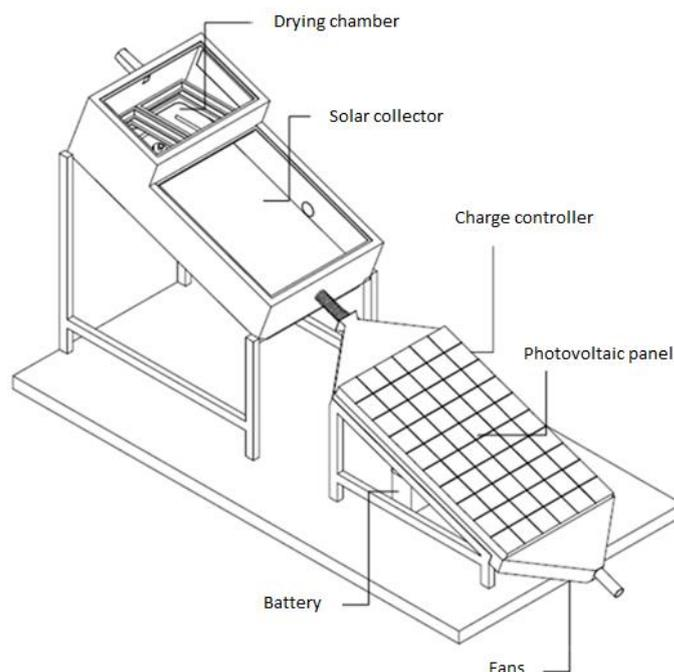
Figure 1. Solar drying system
