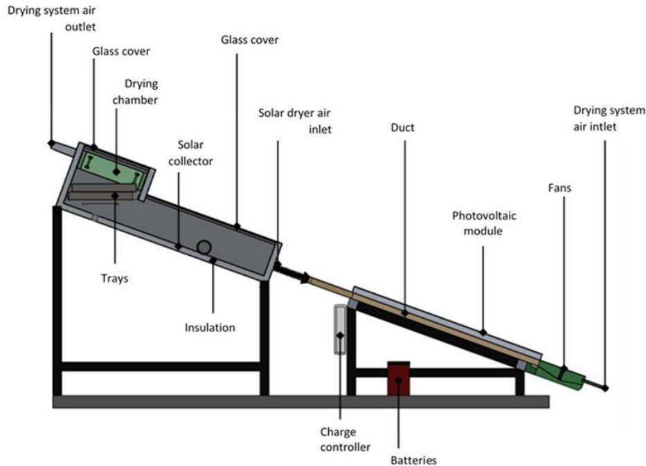
Figure 2. Operation diagram of the drying system
