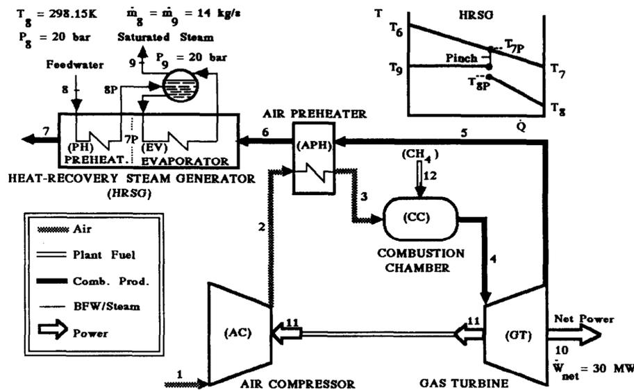
Figure 3. CGAM cogeneration cycle (Valero et al., 1994).
