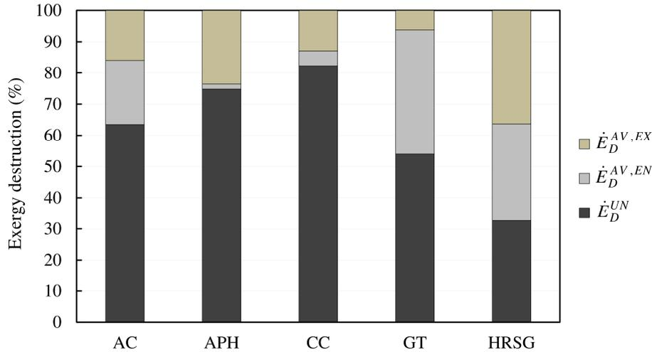
Figure 6. Percentage distribution of the exergy destruction splitting for the  $k$ -th component of the simulated CGAM cycle.
