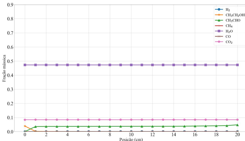
Figure 4. Species mass fractions along the microchannel. System simulated with exhaust gas recirculation of 3%
