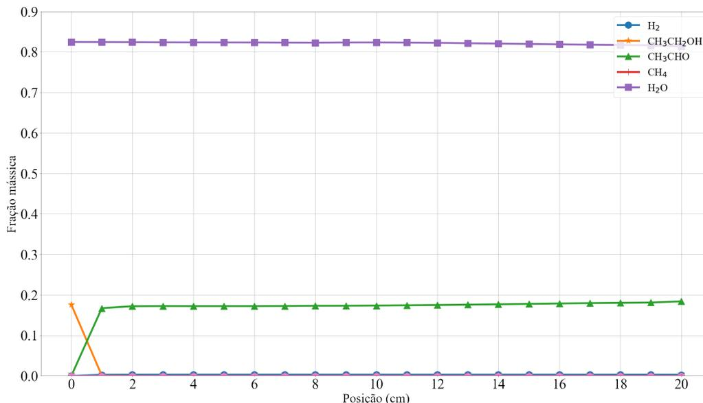
Figure 3. Species mass fractions along the microchannel. System simulated without exhaust gas recirculation
