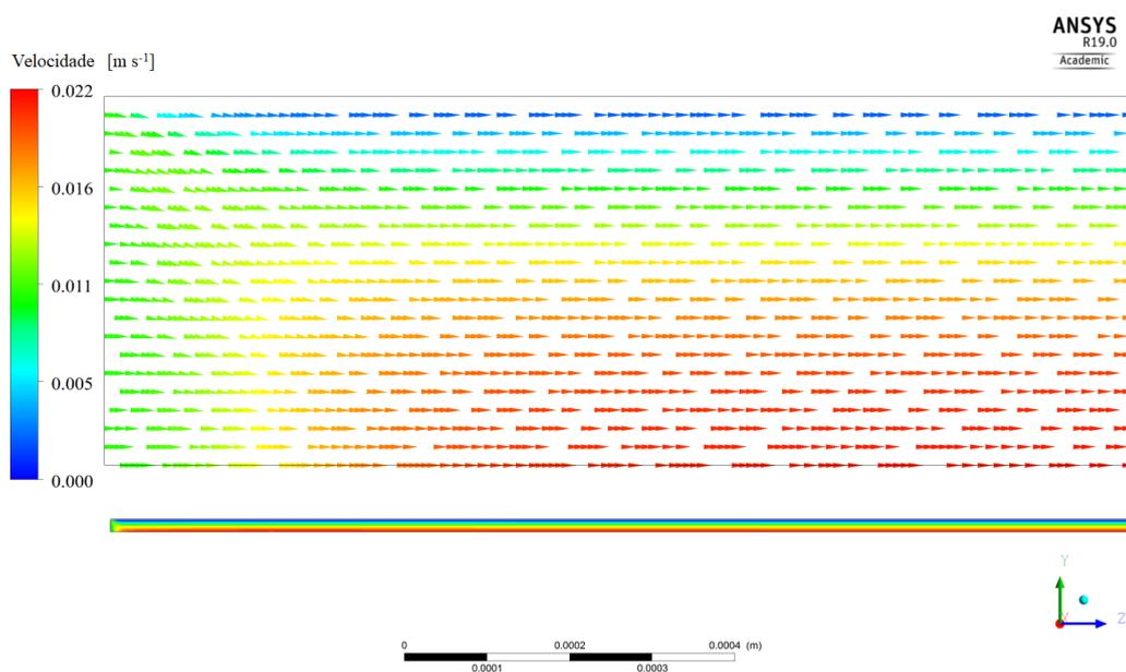
Figure 7. Vector plot of velocity magnitude at inlet region of the channel. System simulated without exhaust gas recirculation
