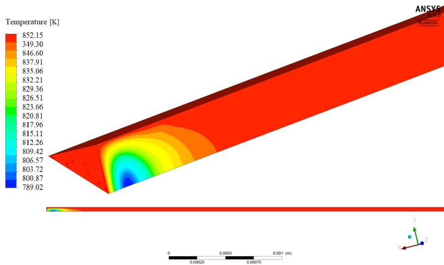
Figure 5. Temperature profile at the symmetry, wall and inlet faces. System simulated without exhaust gas recirculation
