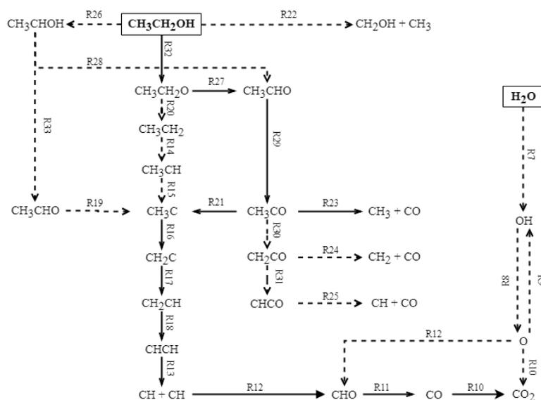
Figure 2. Surface reaction mechanism for steam reforming of ethanol over Nickel. The continuous lines represent the main pathway and the dashed lines represent the alternative pathway. Adapted from (Catapan, 2012)
