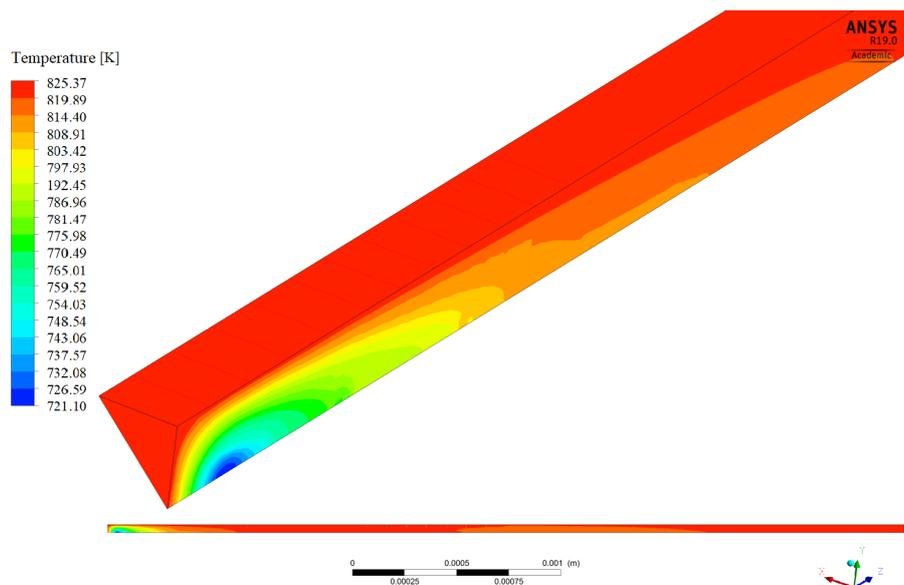
Figure 6. Temperature profile at the symmetry, wall and inlet faces. System simulated with exhaust gas recirculation of 3%.
