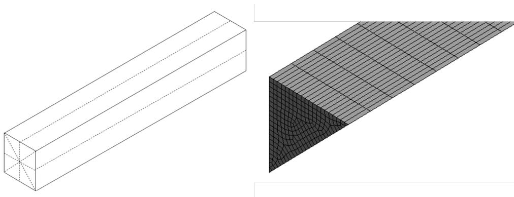
Figure 1. Geometry of the catalytic converter microchannel and the mesh used in simulations.
