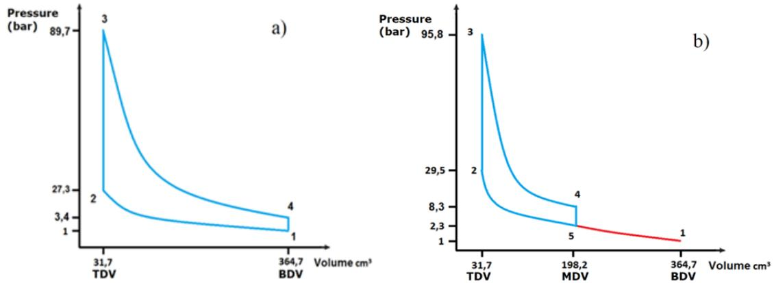
Figure 1. Ideal Otto standard air cycle: a) four-stroke engine; b) two-stroke engine.
