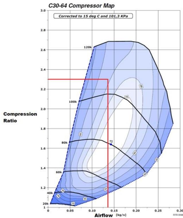
Figure 5. Efficiency map of supercharger C30-64. Adapted from (Rotrex, 2016).
