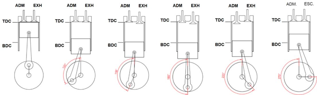
Figure 4. Position of the valves. Start on fuel ignition and gas expansion.
