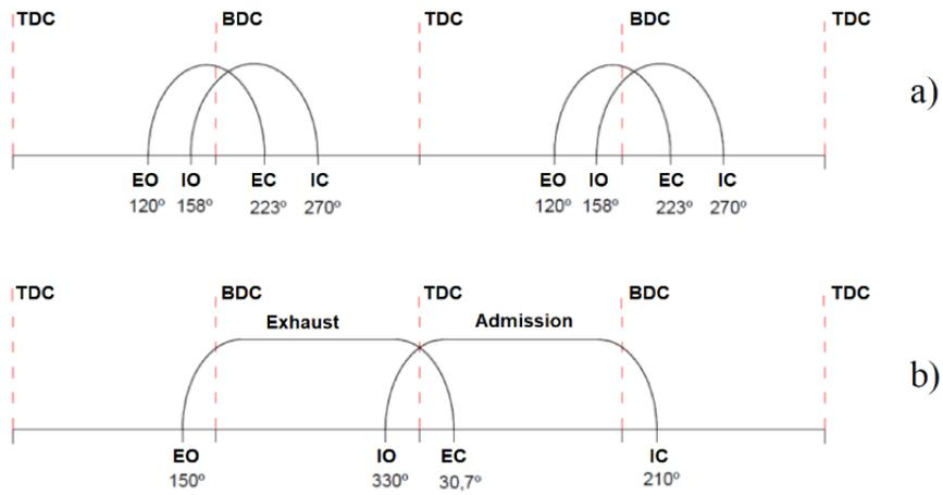
Figure 3. Crankshaft angles for closing and opening valves a) 2-stroke; b) 4 strokes.
