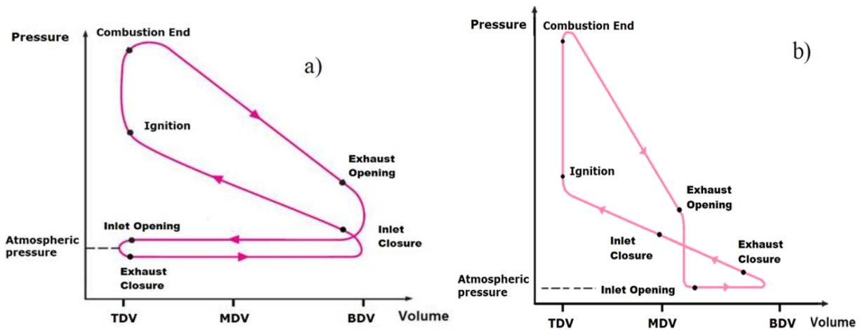
Figure 2. Real cycle: a) four-stroke engine, adapted from (Çengel, 2006). b) two-stroke engine.
