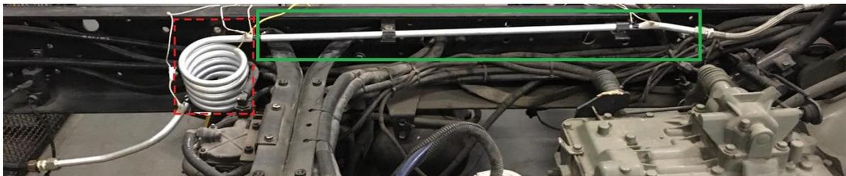
Figure 4. Representation of the steel heat exchanger with the linear control volumes (continuous line) and the control volume of the coil (dashed line) with 5 volutes. (Source: Prepared by the author).
