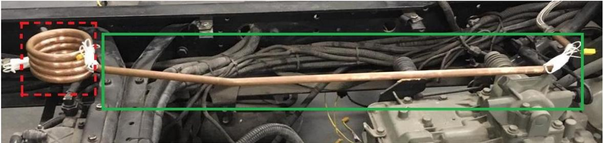
Figure 2. Representation of the copper heat exchanger with linear control volumes (continuous line) and 4-volute “coil” control volume. (Source: Prepared by the author).
