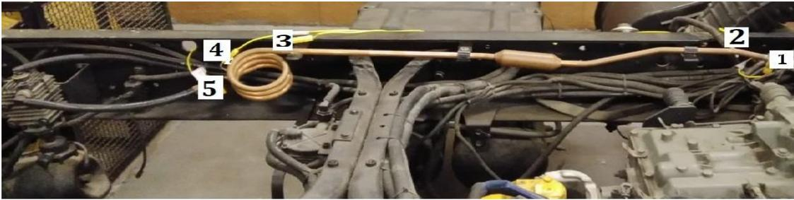
Figure 6. Heat exchanger with the following instrumentation points: 1-Cold Inlet Fluid Temperature ( $T_f$ , e); 2-Inlet Hot Fluid Temperature ( $T_q$ , e); 3-Temperature of Hot Fluid Before Coil; 4-Outflow Hot Temperature ( $T_q$ , s) and 5-Outflow Cold Temperature ( $T_f$ , s).
