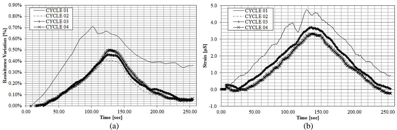
Figure 8 – Measurement results for specimen #3 for four loading-unloading cycles: (a) CNT B; (b) video gauge (after noise filtering).
