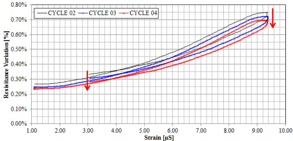
Figure 10 – Resistance variation of CNT A versus strain measured with the metallic foil strain-gauge.
