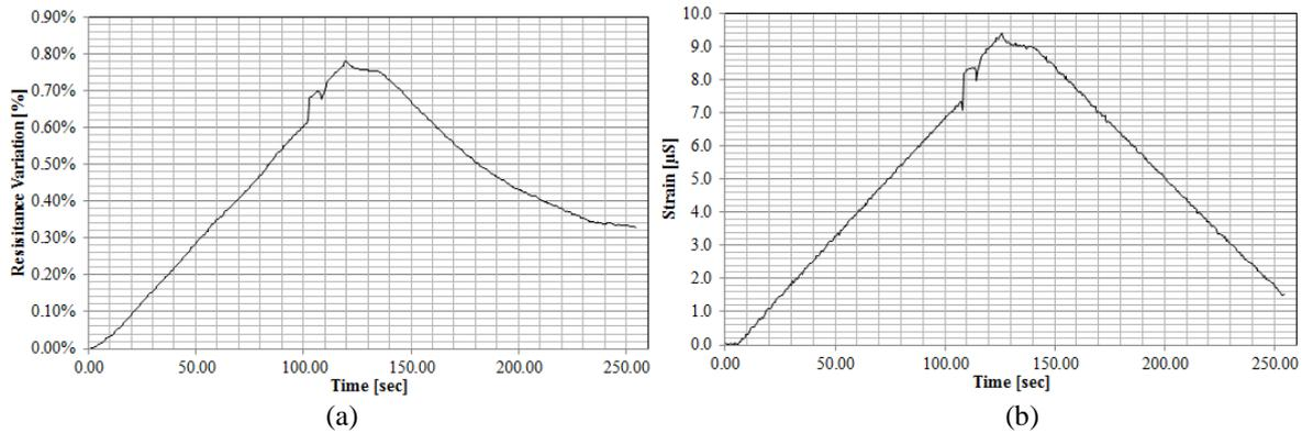
Figure 5 – Measurement results for specimen #3: (a) CNT A; (b) metallic foil strain-gauge.
