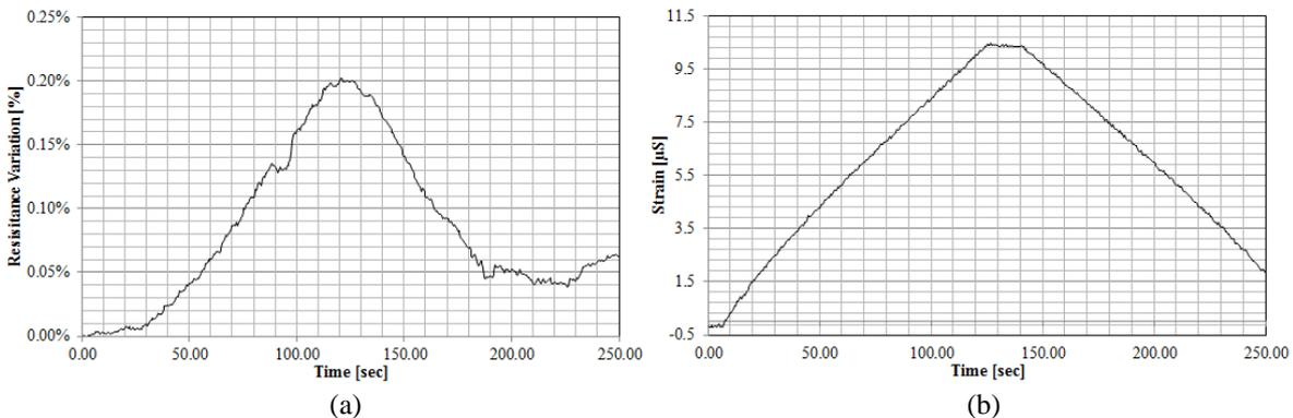
Figure 6 – Measurement results for specimen #2: (a) CNT A; (b) metallic foil strain-gauge.
