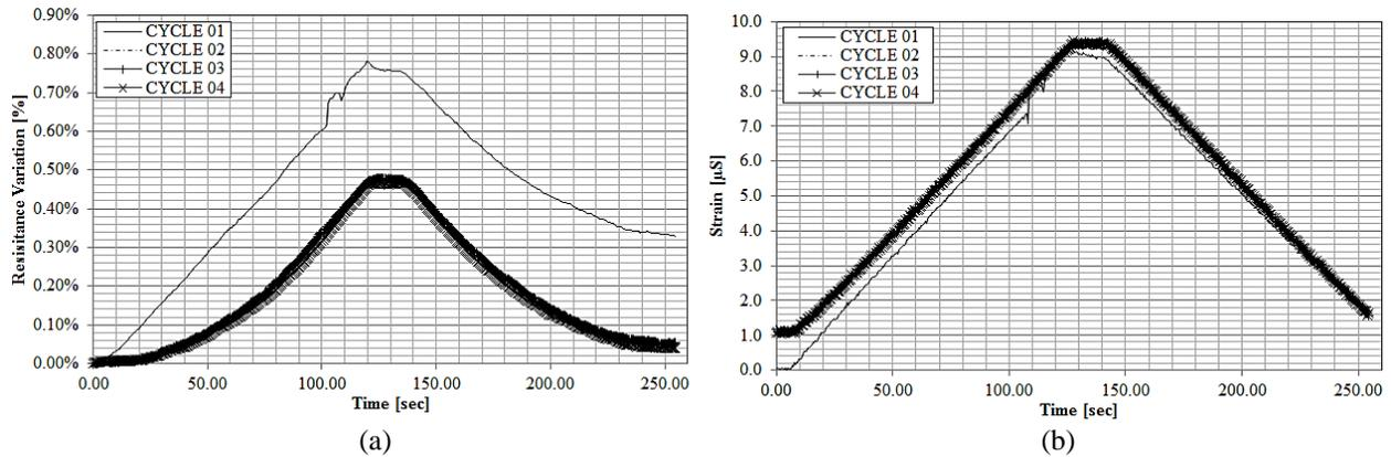
Figure 7 – Measurement results for specimen #3 for four loading-unloading cycles: (a) CNT A; (b) metallic foil strain-gauge.
