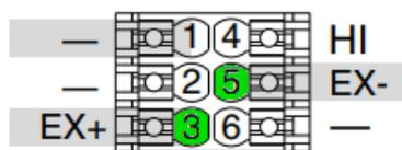
Figure 4 – Half-bridge pin-out
