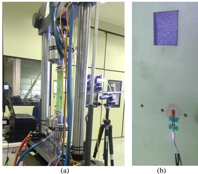
Figure 3 - (a) Illustration of experimental setup; (b) Details of the metallic foil strain-gauge and video gauge sensors
