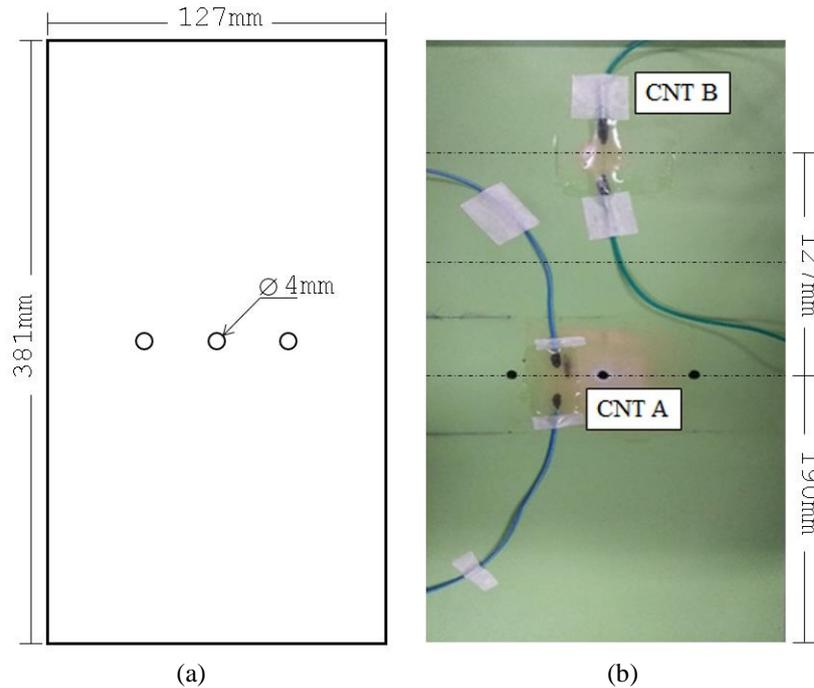
Figure 2: (a) – Illustration and dimensions of Al 2024 T761 plate- thickness of 2.3mm; (b) CNT fibers laminated on an Al 2024-T761 plate.
