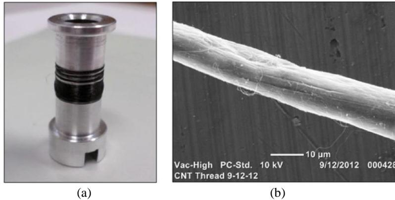
Figure 1: (a) Illustration of a CNT fiber in a spool; (b) scanning electron microscopy of the CNT fiber (Abot *et al.*, 2014).
