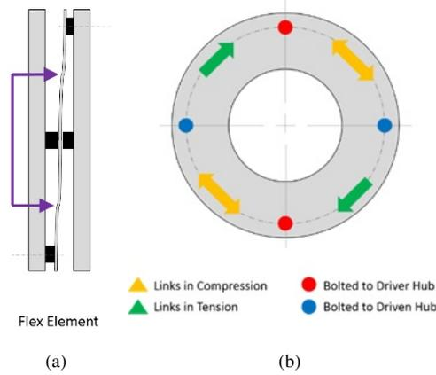
Figure 2. . Disc coupling (a) misalignment accommodation and (b) torque transmission Tuckmantel and Cavalca (2019)
