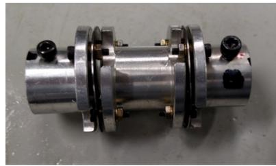
Figure 3. Disc coupling.
