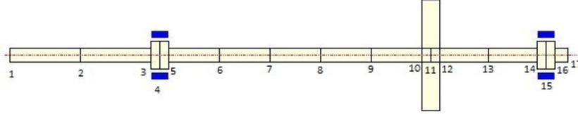
Figure 1. Mathematical model of the rotor.
