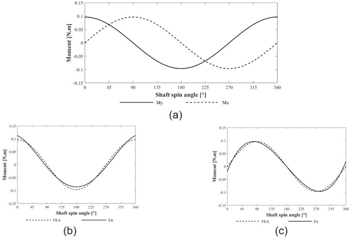
Figure 4. Coupling restoring (a) moments for  $0.5^\circ$  angular misalignment at 20Hz; calculated and adjusted moments (b)  $M_y$  and (c)  $M_z$ .
