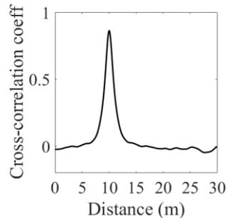
The difference between the above CCC and the one shown in Fig. 6 are the wobbles present in the data, which is due to the leak characteristics. However, the peak is still located at 10 meters, which is the distance from sensor 1 to the leak.
