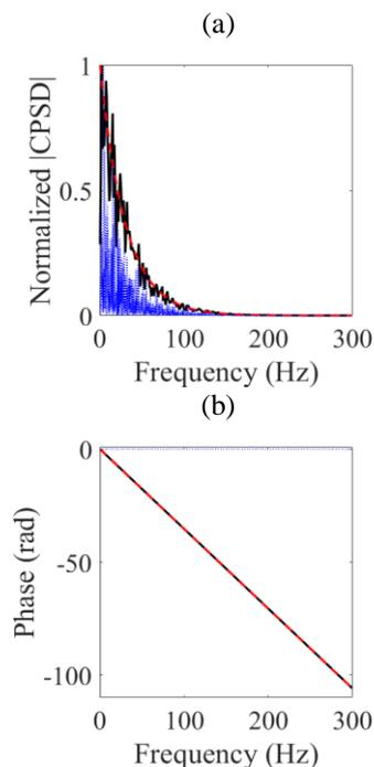
It is observed that the Welch's method smooths the  $|CPSD|$ , enhance the shape when the average is increased, however, reducing the frequency resolution. A longer time length would sort out the problem with the smoothing for analysis 2. The phase, however, is only affected if no average is taken. Likewise for the case 1, the IFFT of Eq. (10) is
