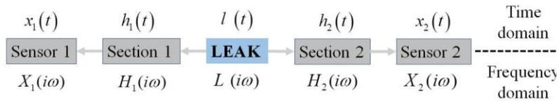
For a better insight into the problem, a simulated leak situation will be performed. This simulation consists in a plastic pipe with the properties given in Tab. 1. The distances  $d_1$  and  $d_2$  are set to 10 m and 30 m, respectively. Figure 3(a) and 3(b) show the modulus and phase for the FRF calculated using Eq.(6) for the pipe Section 1 (black-solid line) and pipe Section 2 (red-dotted line).
