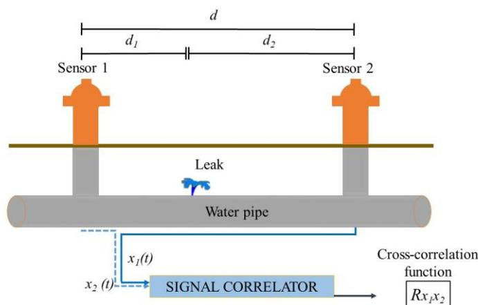
The presence of a leak can be observed as a distinct peak in the cross-correlation function between  $x_1(t)$  and  $x_2(t)$ . The peak in the cross-correlation function occurs at the time delay  $T_0$ , which is the difference in arrival time at both sensors. The leak position can be estimated as (Fuchs and Riehle, 1991)
