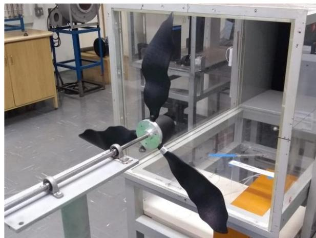
Figure 3: Bench for measuring performance of wind turbines at scale
