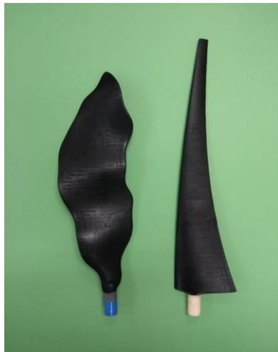
Figure 7: Final scaled model prototypes (conventional and Multiflora blades).
