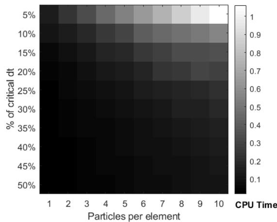
Figure 8: Computation time for a mesh of 3 elements with USL
