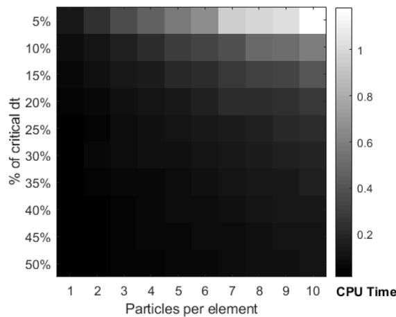
Figure 5: Computation time for a mesh of 3 elements with USF
