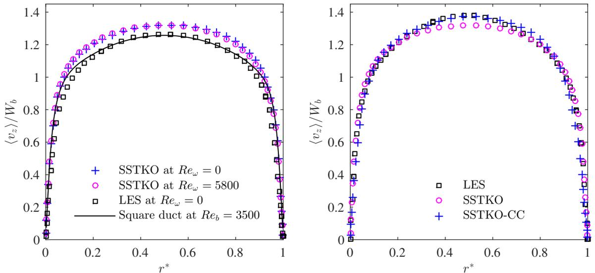
(a) Comparison of SSTKO at  $Re_\omega = 0$  and SSTKO at  $Re_\omega = 5800$  with LES results at  $Re_\omega = 0$  and reference DNS data
