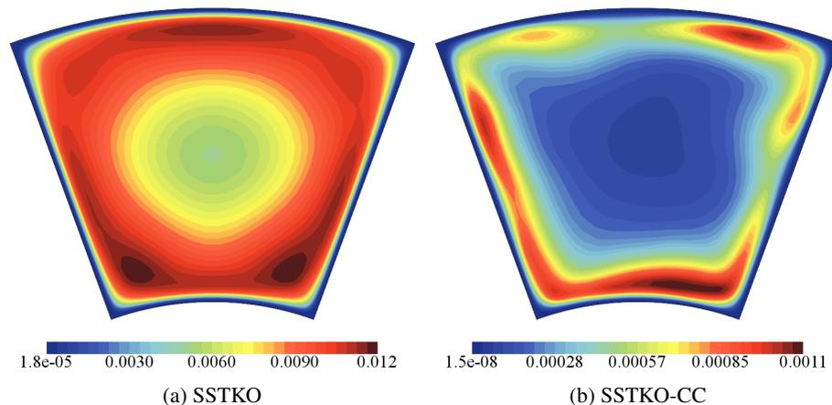
Figure 4: Turbulent kinetic energy scalar field obtained with the (a) SSTKO and (b) SSTKO with curvature correction. The magnitude was normalised by the flow bulk velocity. Rotation direction is clockwise.
