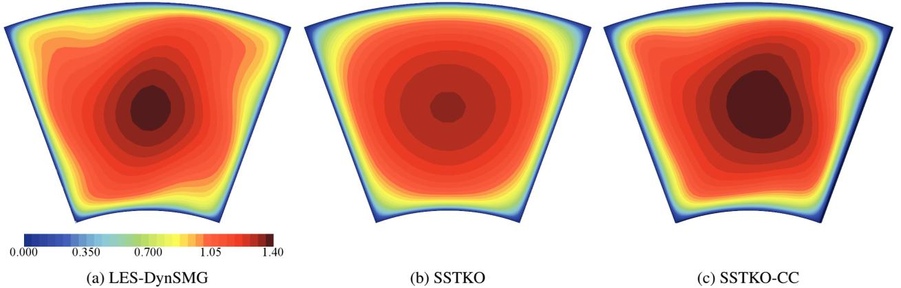
Figure 3: Mean axial velocity field obtained with the (a) LES DynSMG model (b) SSTKO and (c) SSTKO with curvature correction. The velocity magnitude was normalised by the flow bulk velocity. Rotation direction is clockwise.
