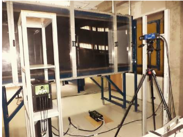
Figure 11: PIV system installed in the wind-tunnel test-section.
