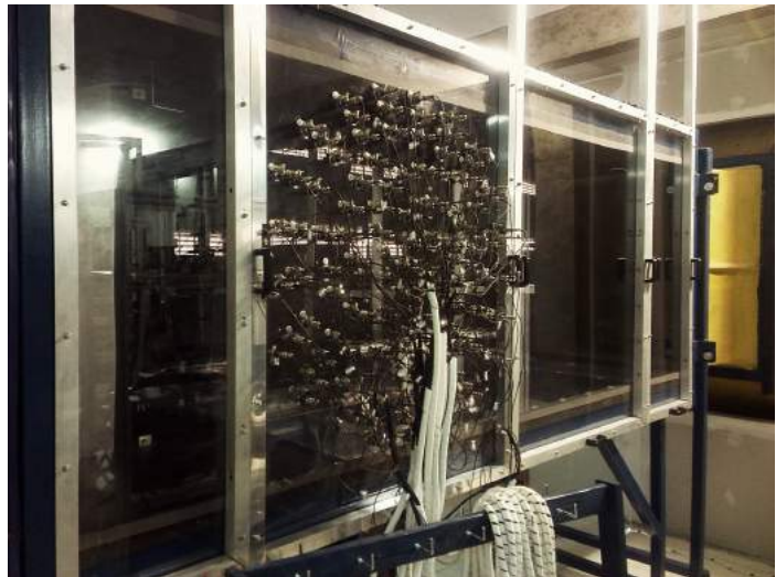
(b) Antenna mounted on the test-section window
