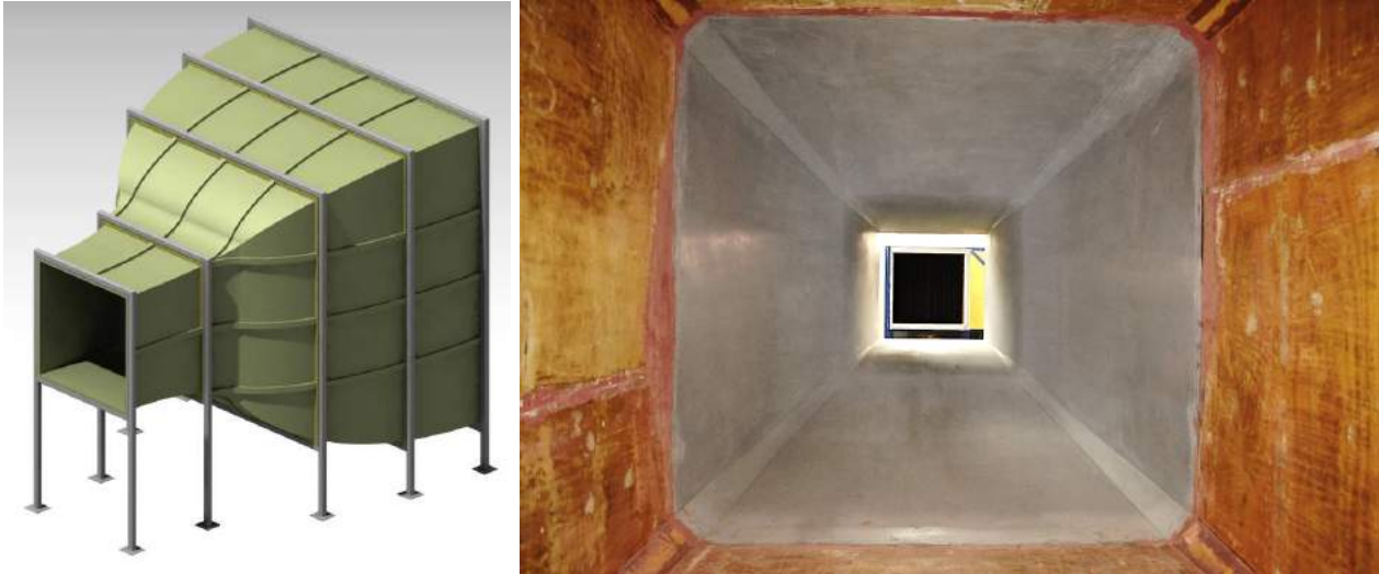
(a) Contraction design (b) Contraction picture taken from the inside of the settling chamber Figure 8: Contraction employed to induce a flow acceleration from the settling chamber to the test-section.
