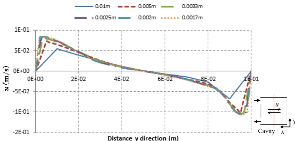
Figure 2. Variation of velocity  $u$  along the  $y$  direction (for  $x = L/2$ ) for different mesh sizes.
