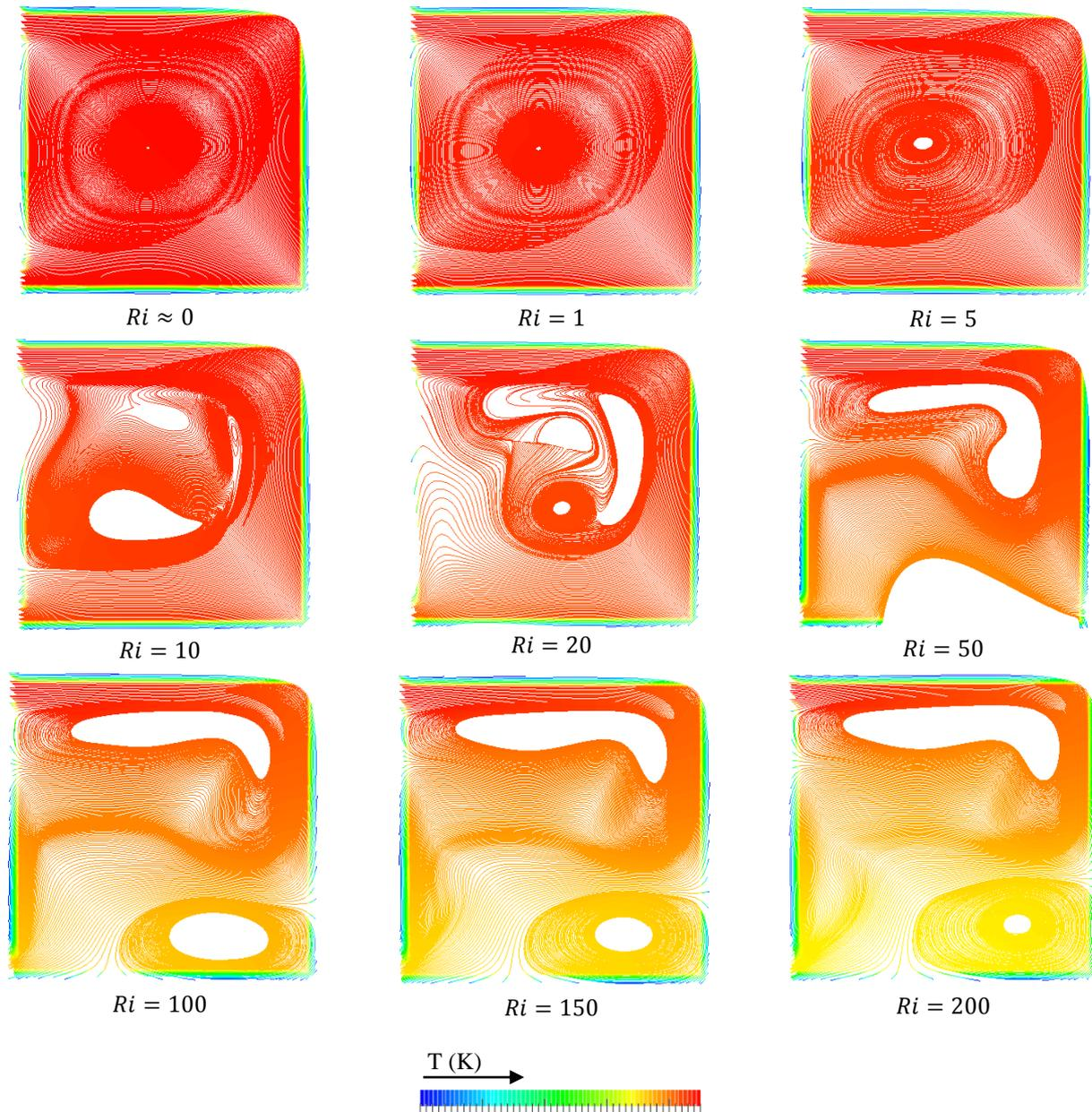
Figure 5. Streamlines with temperature profiles for different Richardson numbers.
