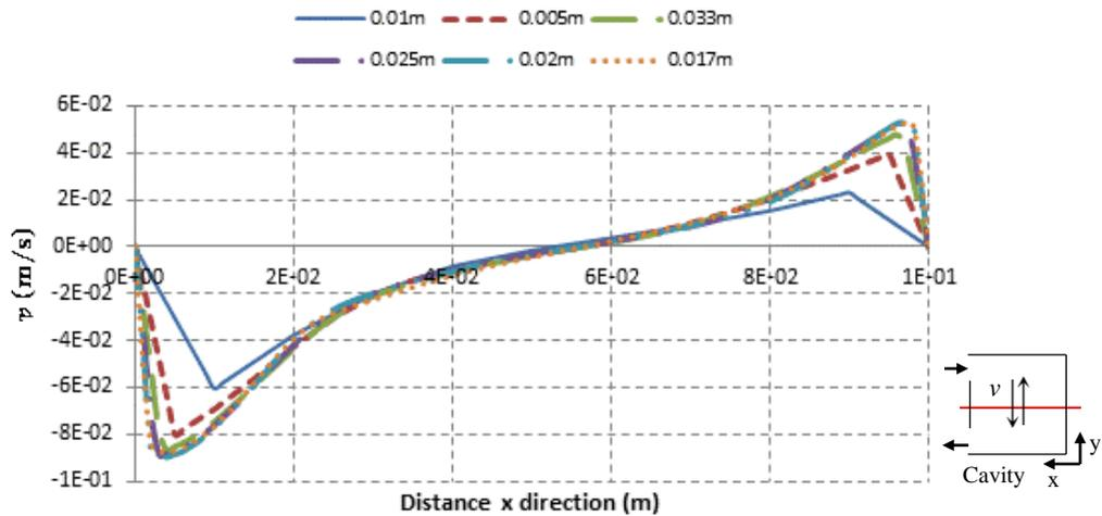
Figure 3. Variation of velocity  $v$  along the  $x$  direction (for  $y = H/2$ ) for different mesh sizes.
