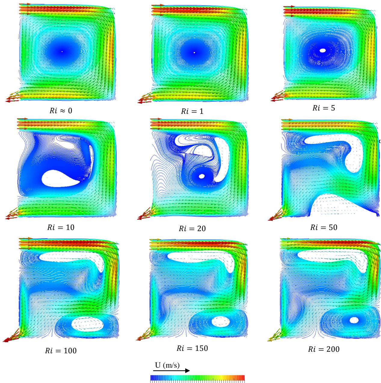
Figure 4. Streamlines with velocity profiles for different Richardson numbers.
