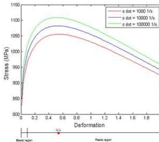
**Figure 1.** Stress-strain curve of AISI 1045 steel for three strain rates (Scaduto & Menezes, 2016).
