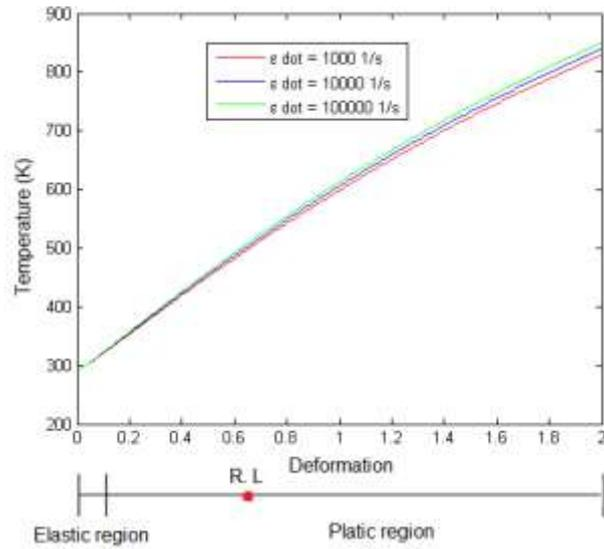
**Figure 8.** Temperature variation with the deformation of AISI 4340 Steel for three different high strain rates (Scaduto & Menezes, 2016).
