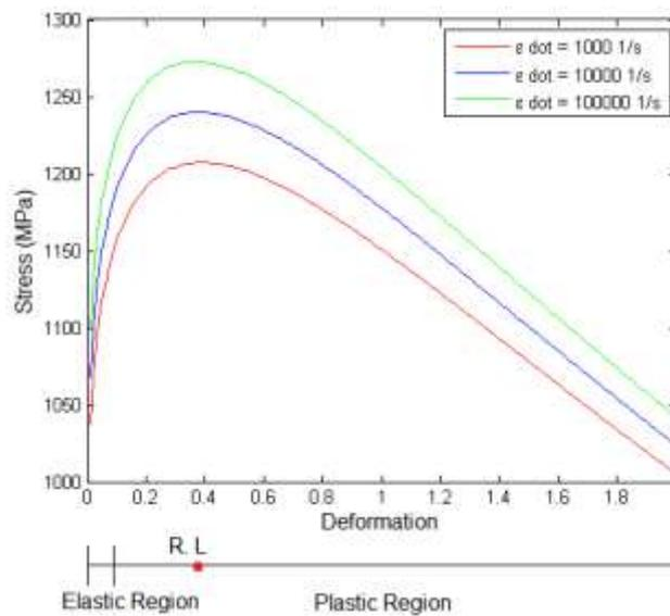
**Figure 7.** Stress-strain curves of AISI 4340 steel for three different high strain rates (Scaduto & Menezes, 2016).
