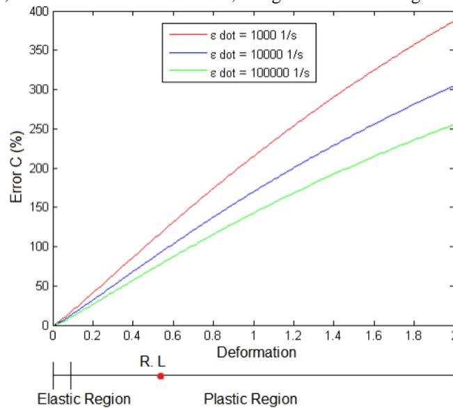
**Figure 11.** Error variations of the parameter  $C$  for AISI 4340 Steel comparing the value obtained by the method with those proposed in the literature for each level of deformation at three different high strain rates (Scaduto & Menezes, 2016).
