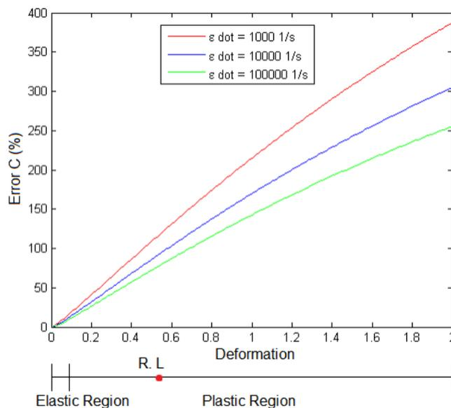
**Figure 5.** Error variation of the parameter  $C$  for AISI 1045 Steel comparing the value obtained by the method proposed with that found in the literature for each level of deformation for three different high strain rates (Scaduto & Menezes, 2016).
