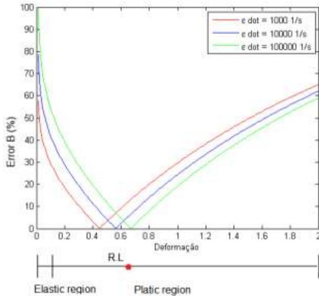
**Figure 10.** Error variations of the parameter  $B$  for AISI 1045 Steel by comparing the value obtained by the method proposed in the literature for each level of deformation at three different high strain rates (Scaduto & Menezes, 2016).
