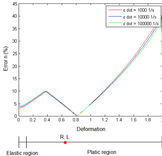
**Figure 9.** Error variations of the parameter  $n$  for AISI 4340 Steel comparing the value obtained by the method proposed in the literature for each level of deformation at three different high strain rates (Scaduto & Menezes, 2016).
