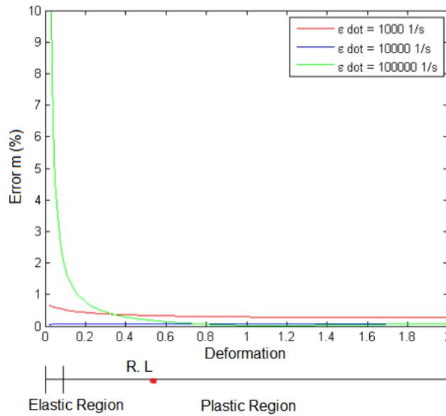
**Figure 6.** Variation of the error of the parameter  $m$  for AISI 1045 Steel comparing the value obtained by the method proposed with that found in the literature for each level of deformation for three different high strain rates (Scaduto & Menezes, 2016).
