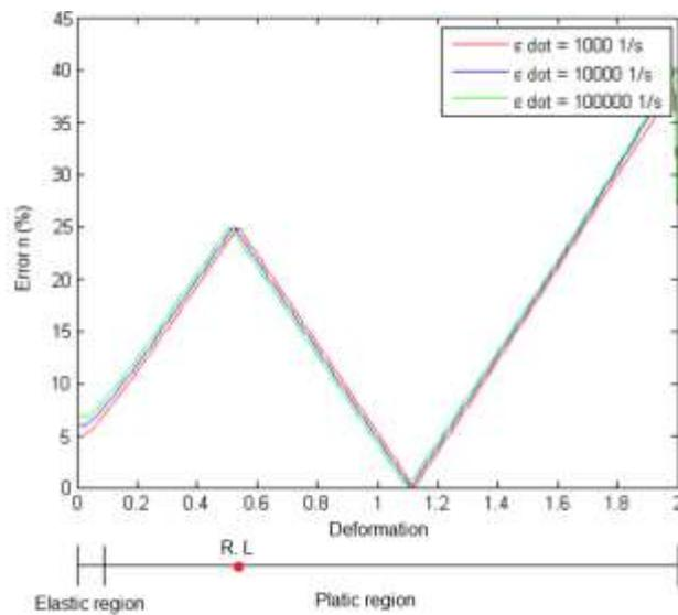
**Figure 3.** Error variation of the parameter  $n$  for AISI 1045 Steel comparing the value obtained by the method proposed with that found in the literature for each level of deformation for three strain rates (Scaduto & Menezes, 2016).
