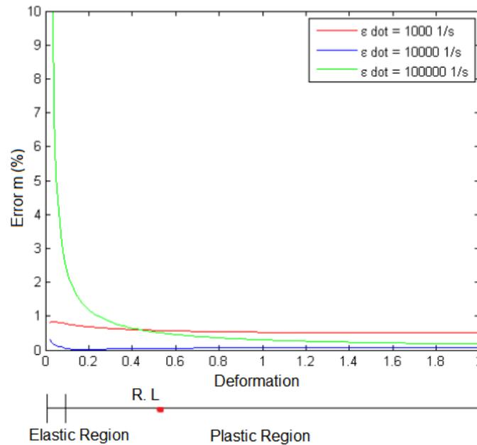
**Figure 12.** Error variations of the parameter  $m$  for AISI 4340 Steel comparing the value obtained by the method with those proposed in the literature for each level of deformation at three different high strain rates (Scaduto & Menezes, 2016).
