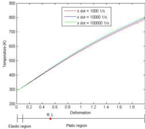
**Figure 2.** Temperature variation with the deformation of AISI 1045 Steel for three strain rates (Scaduto & Menezes, 2016).
