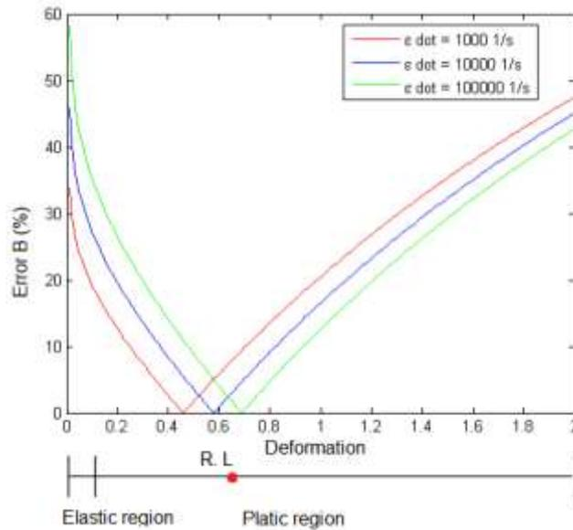
**Figure 4.** Error variation of parameter  $B$  for AISI 1045 Steel by comparing the value obtained by the method proposed with that found in the literature for each level of deformation for three different high strain rates (Scaduto & Menezes, 2016).
