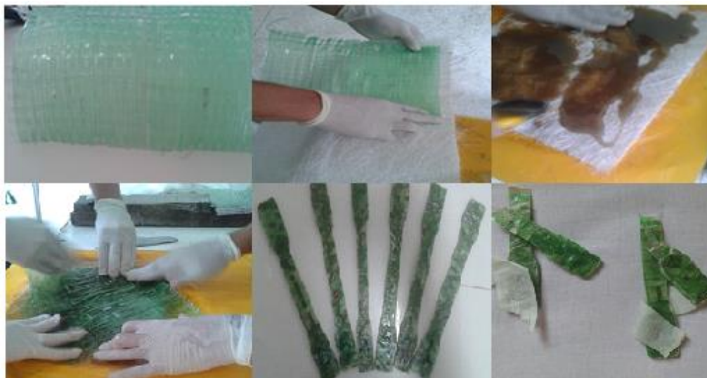
Figure 1. (a) PET Blanket interlaced; (b) Cutting the fiberglass; (c) Application of the resin in the fiberglass; (d) PET, resin and PET at a 45 ° angle; (e) Samples; (f) Samples after tensile test.
