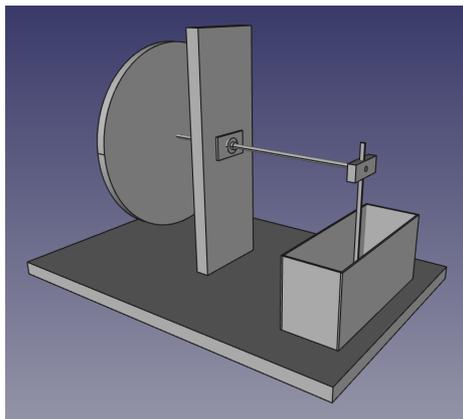
Figure 8. Bench design with viscous friction
