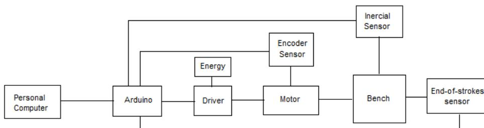
Figure 10. Instrumentation diagram
