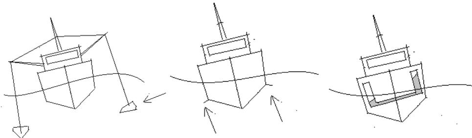
Figure 2. (a) Paravanes (b) BilgeKeels (c) U-Tank stabilization
