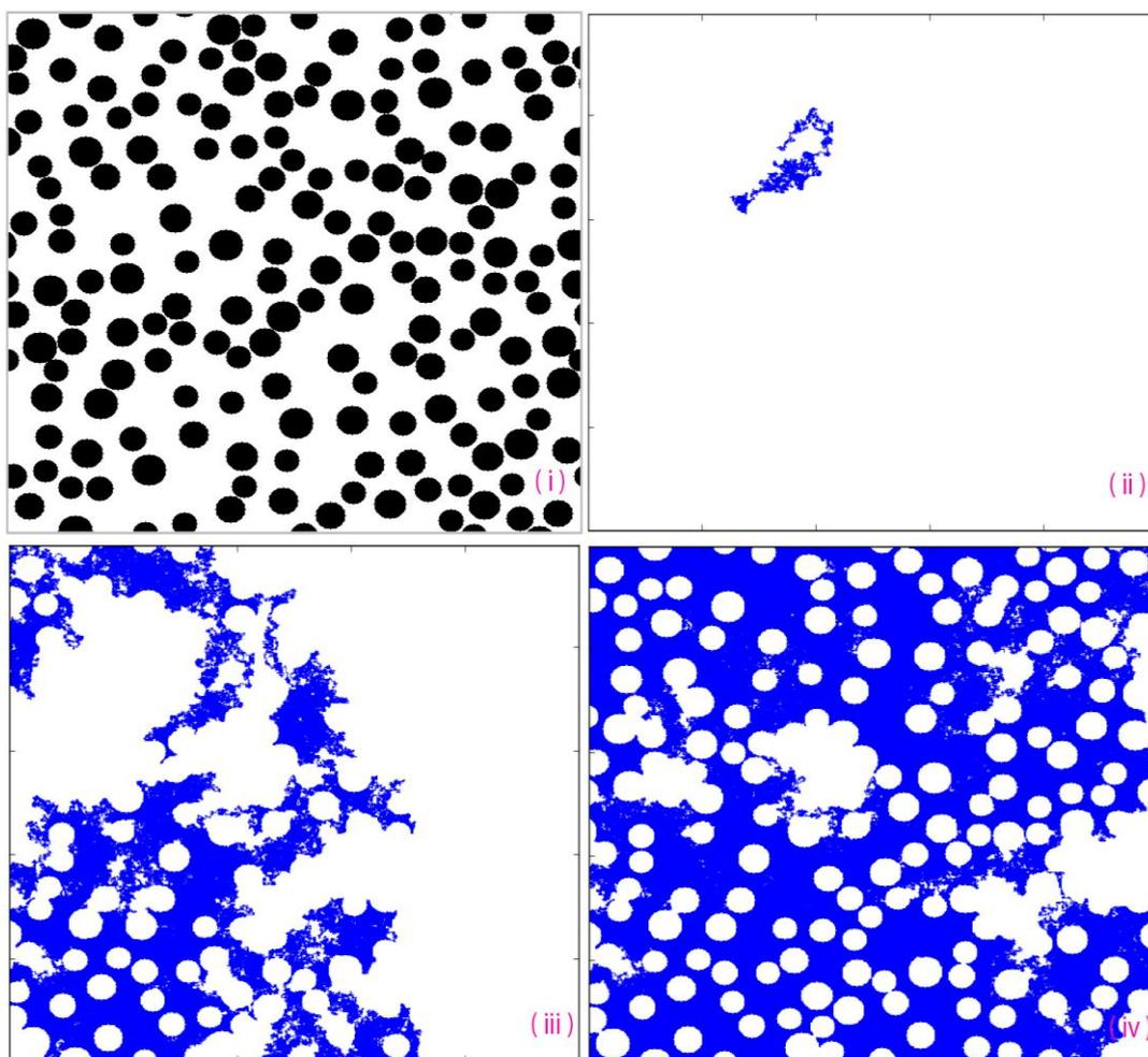
Figure 1. Example 2D of Random Walk. (i) artificial 2D geometry where the black represents the solid parts and white pore. (ii) to (iv) path evolution of a walker in relation to the number of steps.
