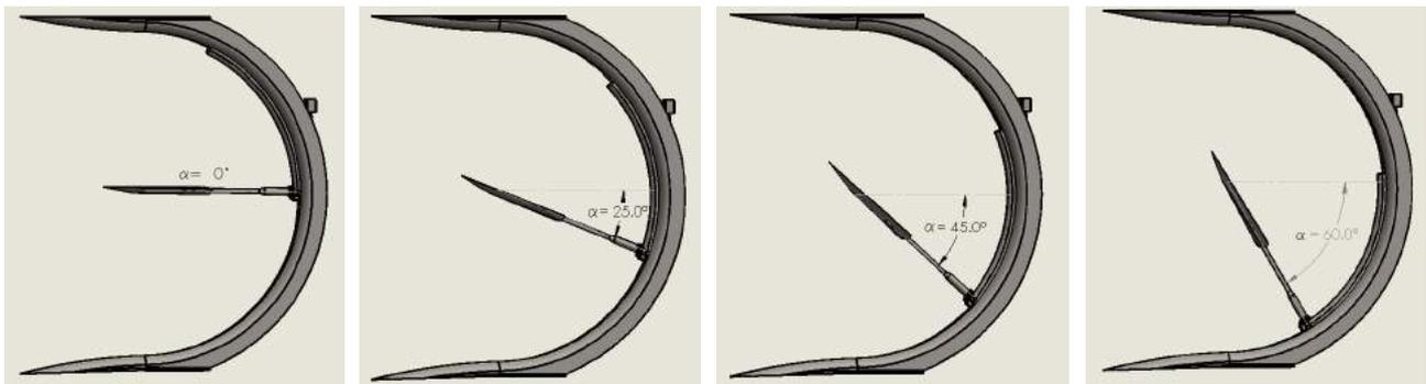
Figure 6: Proposed design of the device to perform roll cycle limit oscillations.
