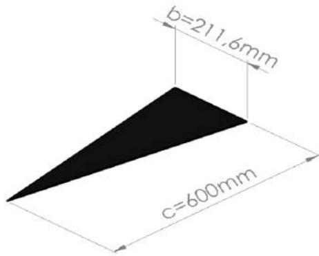
(a) Representation of delta wing model with  $\Lambda = 80^\circ$  and its main dimensions.
