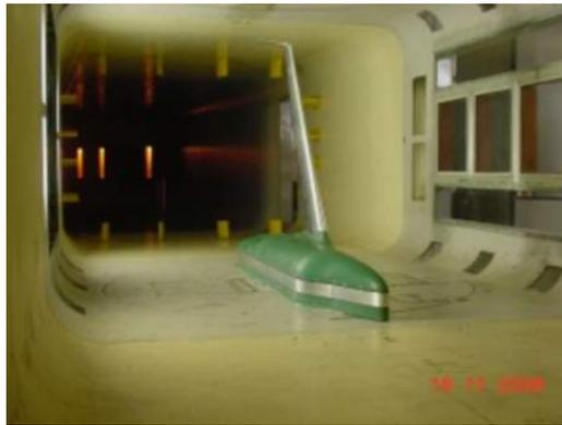
Figure 3: Test section of wind tunnel TA-02 at Brazilian Institute of Aeronautics (IAE).
