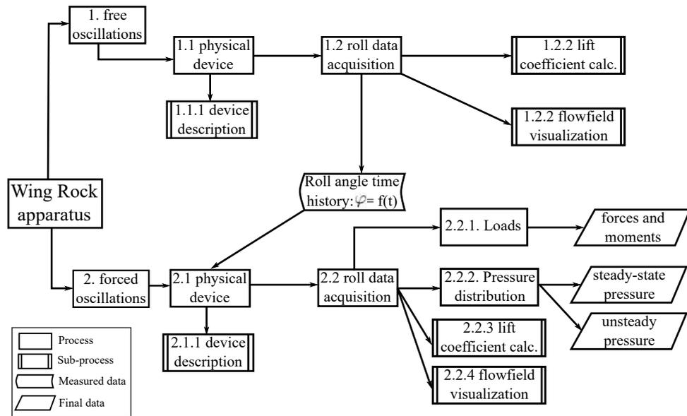
Figure 5: Representation of the apparatus architecture with the experiment strategy. Besides the physical device, the flow visualization techniques and instrumentation hardware are necessary.
