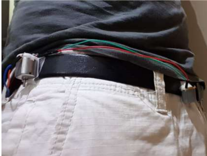
Figure 8 - Belt with micro motors.
