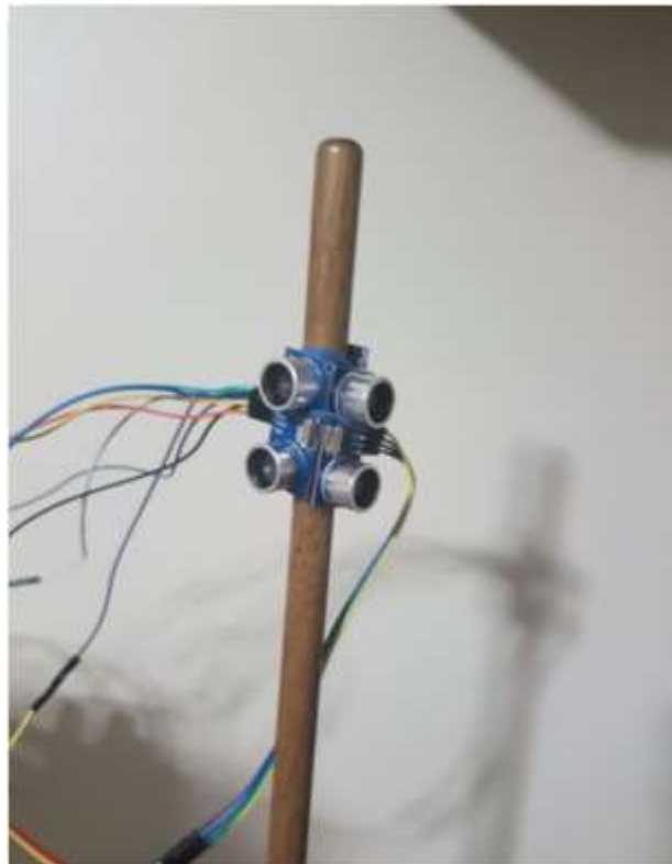
Figure 9 - Drumstick with ultrasonic sensors.
