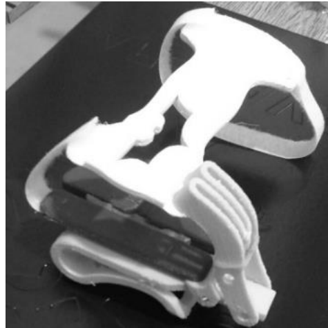
Figure 9. Orthosis' mock-up (generated by FDM technique)
