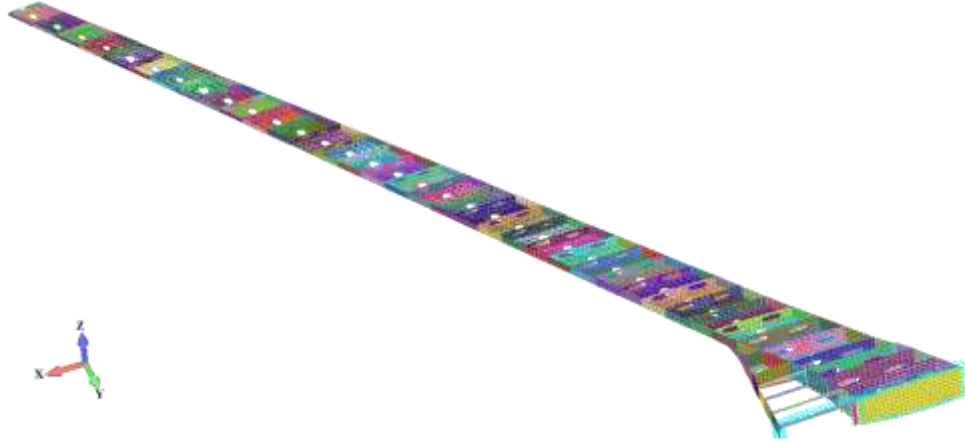
Figure 1. Wing box structural layout
